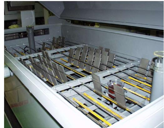
FIG. 13. Combined Cyclic Corrosion Test Instrument
