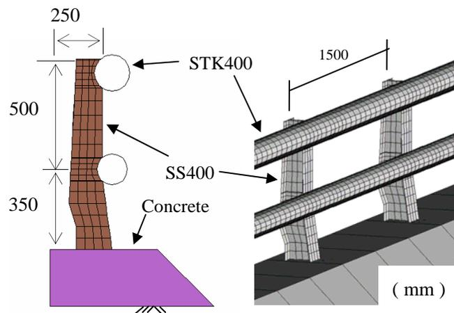
Figure 9: Model of steel guard fence
