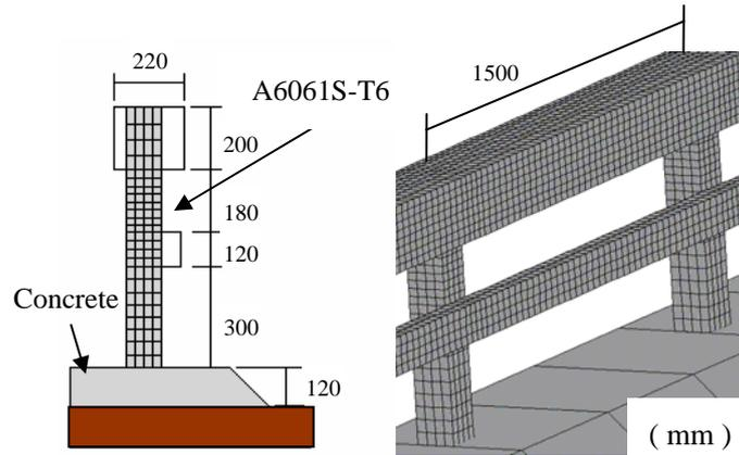
Figure 10: Model of aluminum alloy guard fence
