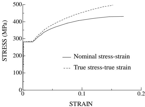
Figure 1: Stress-strain relationship of SS400
