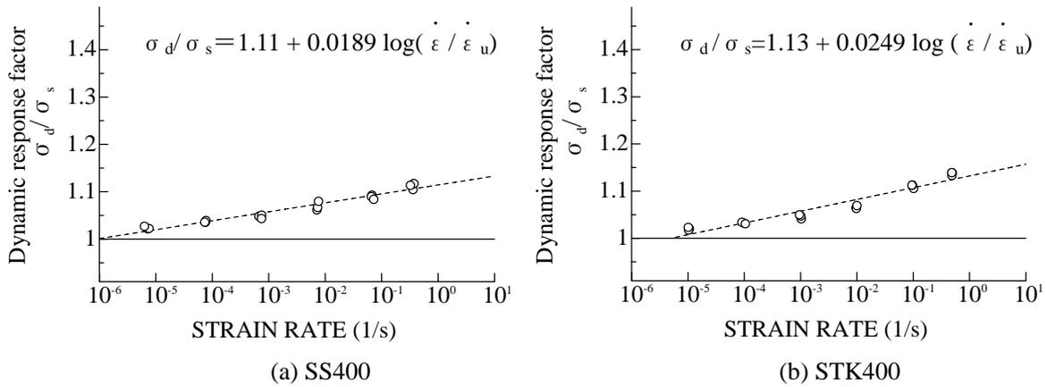
Figure 4: Strain rate effects on ultimate stress
