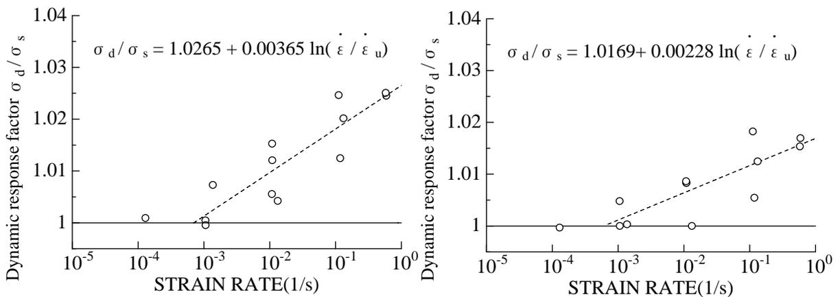
Figure 6: Strain rate effects on yield stress
