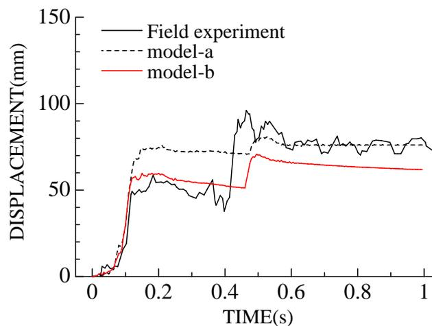
Figure 11: Numerical analysis result of steel guard fence
