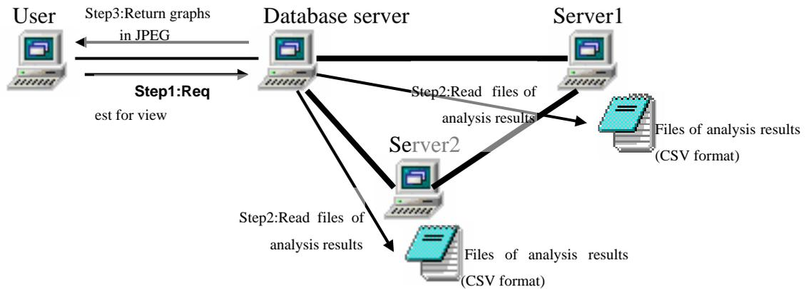
Fig. 6: The function of drawing graphs
