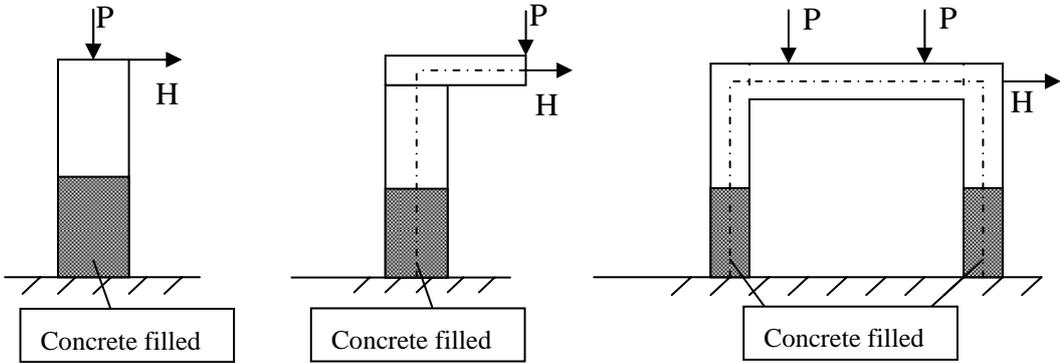
Fig. 1: The models of static analysis
