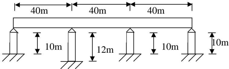
Fig. 3: The model of time-history response analysis of continuous bridge structure
