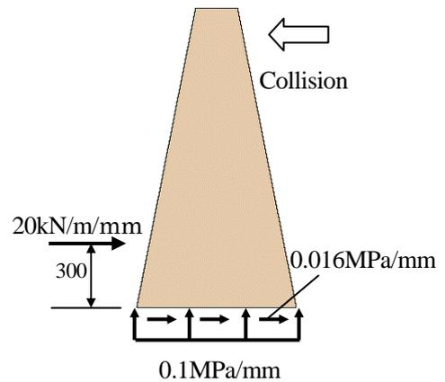
Figure 2. Subgrade spring model
