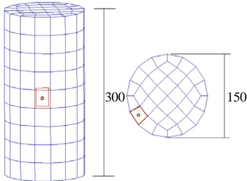
Figure 5. Concrete test specimen model (unit : mm)
