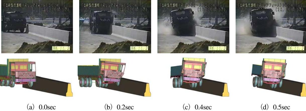
Figure 9. Vehicle behaviors compared with the field collision experiment results
