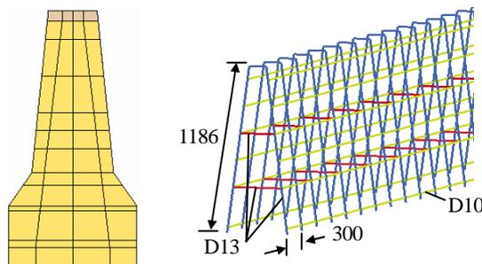
(a) Concrete body (b) Arrangement of reinforcing bars
