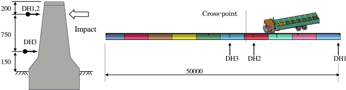
Figure 10. The location points of measured displacement
