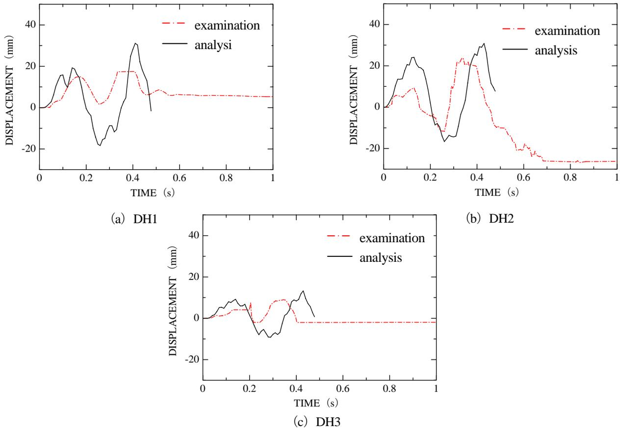
Figure 11. The response displacement of concrete guard fence
