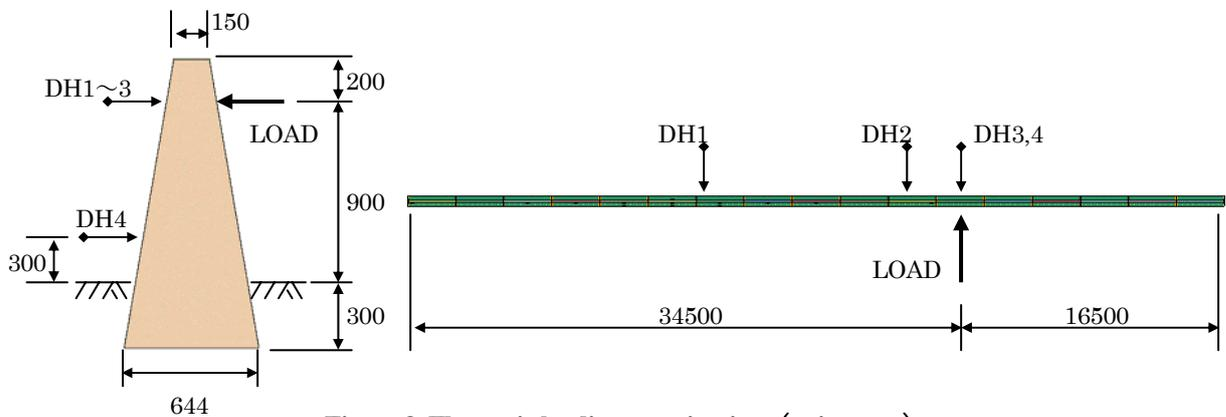
Figure 3. The static loading examination (unit : mm)
