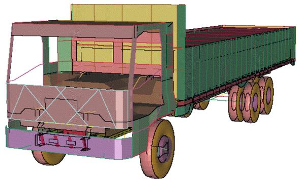
Figure 8. The FEM model of vehicle
