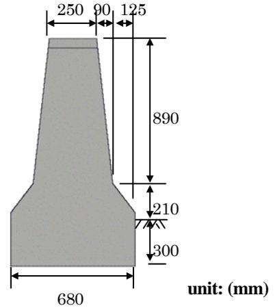
Figure 1. Florida type concrete guard fence
