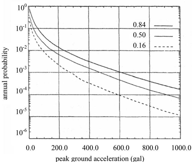
Figure 1. Fractal seismic hazard curves.
