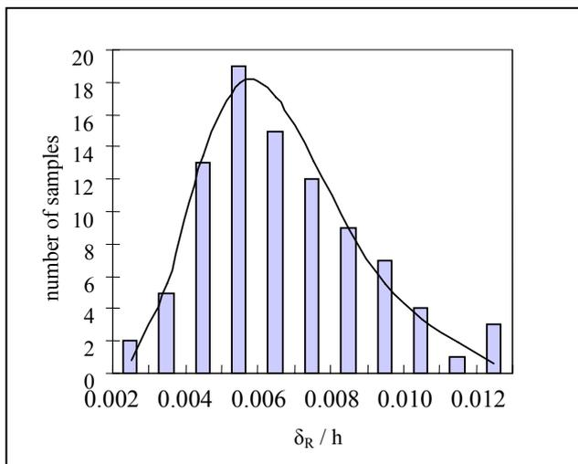
Figure 4. Histogram of residual displacement.
