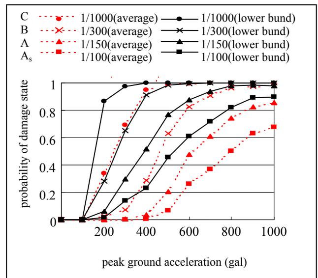
Figure 5. Fragility curves of steel bridge piers.
