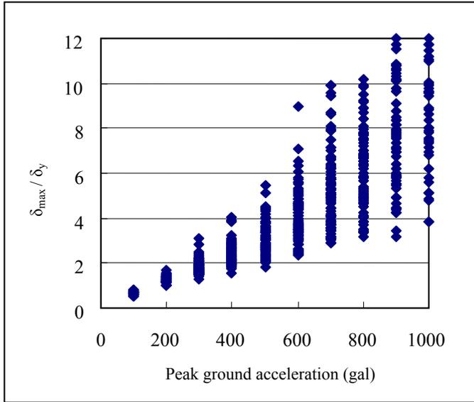
Figure 2. Maximum response displacements.
