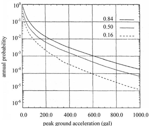
Figure 1. Fractal seismic hazard curves.
