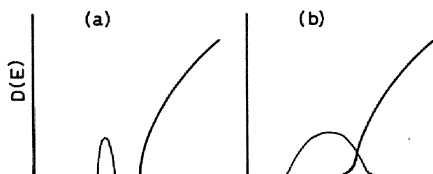
Fig. 5-1. The electronic states in the impurity band may be described by atomic wave functions and should have localized nature, while electrons in the main band behave like free electrons. At a finite temperature electronic properties should reflect both features.
