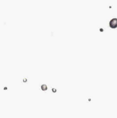
(b) MnS ; weld metal by M3 electrode wire
