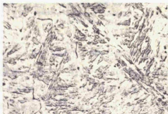
Photo. 4-4 Microstructure of cast specimen containing 0.11% Ti \times 400
