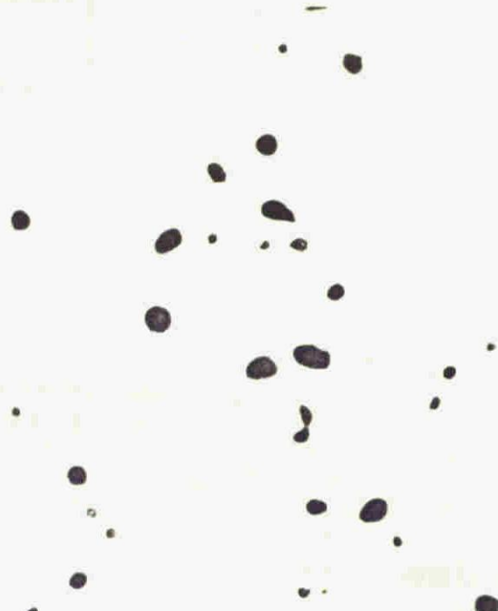
(b) \text{MnS} ; Mn% in weld metal=1.93
