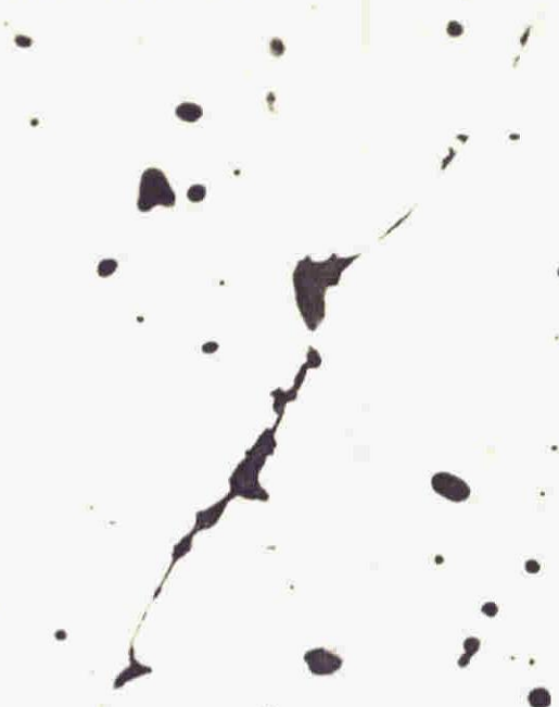
(a) (\text{Fe}, \text{Mn})\text{S} ; Mn% in weld metal=0.49
