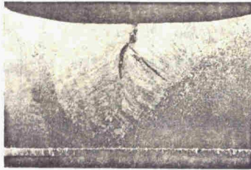
Photo・2-7 Macro-photograph of hot cracking; weld metal by 3.5% Ni steel electrode- wire; \times 3
