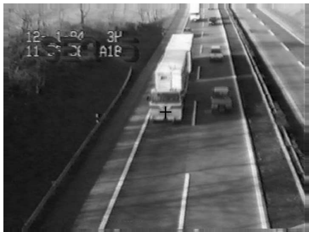
Fig. 2. Scene taken from a highway sequence; the vehicles running on the right lane are shadowed by the vehicle running on the left lane. The data shown in Fig. 1 are collected at the position of the cross.
