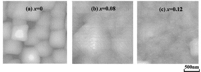
Fig. 2. AFM images of (a) SmBCO film deposited with  $x = 0$ , (b) SmBCO film deposited with  $x = 0.08$  and (c) SmBCO film deposited with  $x = 0.12$ .
