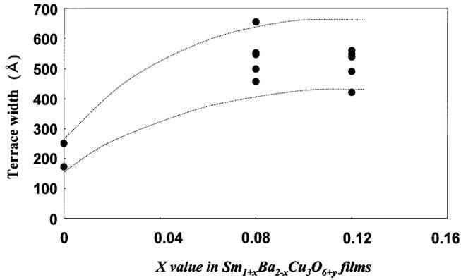
Fig. 4. Dependence of the terrace width on the  $x$  value in  $\text{Sm}_{1+x}\text{Ba}_{2-x}\text{Cu}_3\text{O}_{6+y}$  films on the MgO substrates taken from the AFM images.
