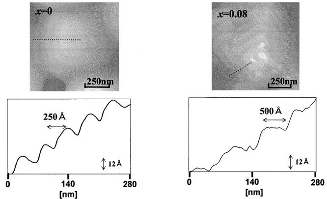
Fig. 3. AFM images and line scan profile of (a) a SmBCO film deposited with  $x = 0$  and (b) a SmBCO film deposited with  $x = 0.08$ .
