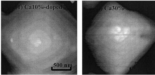
Fig. 5. AFM images of the  $\text{Sm}_{0.9}\text{Ca}_{0.1}\text{Ba}_2\text{Cu}_3\text{O}_{6+y}$  films and the  $\text{Sm}_{0.7}\text{Ca}_{0.3}\text{Ba}_2\text{Cu}_3\text{O}_{6+y}$  films showed in (1) and (2), respectively.
