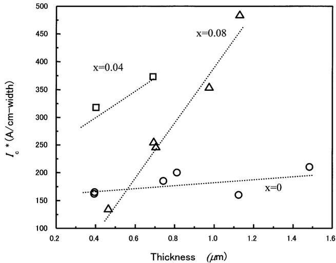
Fig. 1. Projected critical current ( $I_c^*$ ) for 1 cm width as a function of SmBCO film thickness. The open circles, squares and triangles correspond to the data of  $x = 0, 0.04$  and  $0.08$ , respectively.
