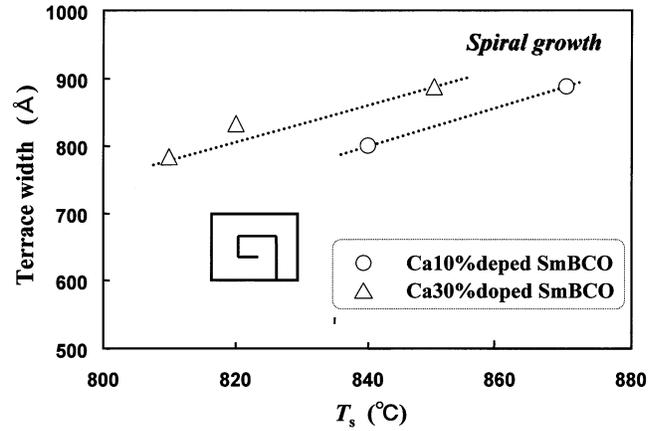
Fig. 6. Dependence of the terrace width on the substrate temperature for (SmCa)  $\text{Ba}_2\text{Cu}_3\text{O}_{6+y}$  films on the MgO substrates from the AFM images. The open circles and triangles correspond to the data of the films fabricated using the  $\text{Sm}_{0.9}\text{Ca}_{0.1}\text{Ba}_2\text{Cu}_3\text{O}_{6+y}$  target and the  $\text{Sm}_{0.7}\text{Ca}_{0.3}\text{Ba}_2\text{Cu}_3\text{O}_{6+y}$  target, respectively.
