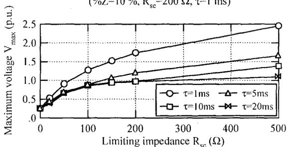
(b) Maximum voltage as a function of limiting impedance
