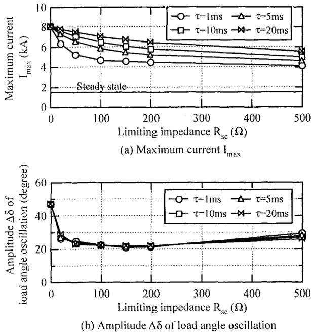
Fig. 4. Maximum current  $I_{max}$  and amplitude  $\Delta\delta$  of load angle oscillation as a function of limiting impedance ( $\%Z=10\%$ ).
