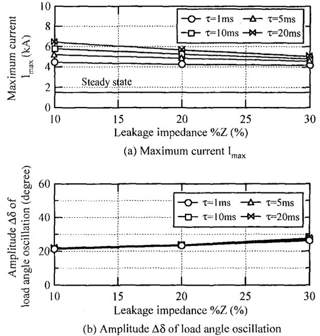
Fig. 5. Maximum current  $I_{max}$  and amplitude  $\Delta\delta$  of load angle oscillation as a function of leakage impedance ( $R_{sc}=200 \Omega$ ).
