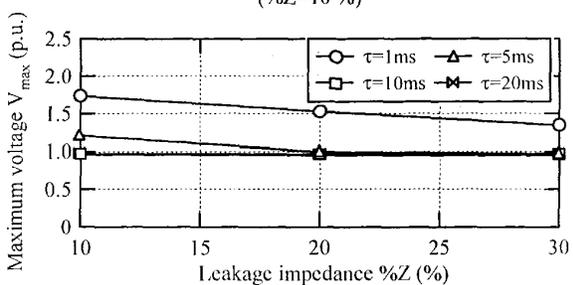
(c) Maximum voltage as a function of leakage impedance
