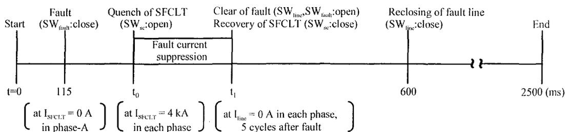
Fig.2. Switching operation and time sequence after fault.
