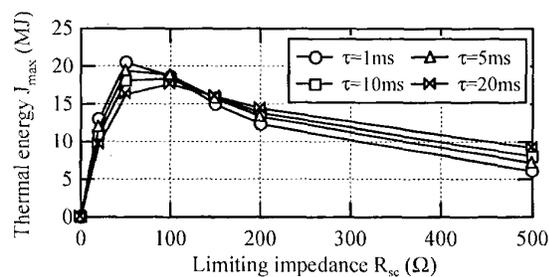
(b) Thermal energy as a function of limiting impedance
