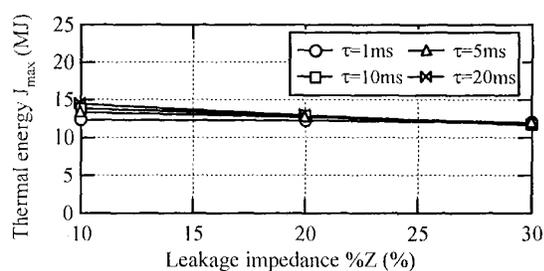
(c) Thermal energy as a function of leakage impedance
