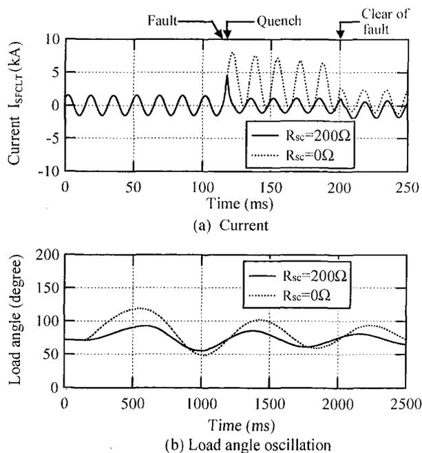
Fig. 3. Current and load angle oscillation ( $\%Z=10\%$ ,  $R_{sc}=200\ \Omega$ ,  $\tau=1\text{ ms}$ ).
