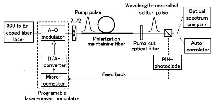
Fig. 1. Experimental setup of electronically controlled high-speed wavelength-tunable femtosecond soliton pulse generation.
