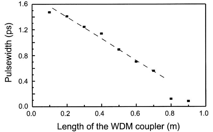
Fig. 3. Observed compressed pulsewidth measured by the autocorrelator as a function of the length of the WDM coupler.
