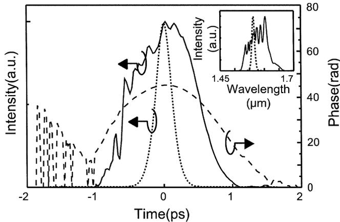
Fig. 2. Temporal and spectral waveform (solid line) and phase (broken line) of the pulses after propagation of normal dispersive EDF. Dotted line represents incident pulses.
