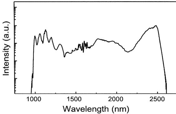
Fig. 5. Optical spectrum of generated ultrabroad SC.
