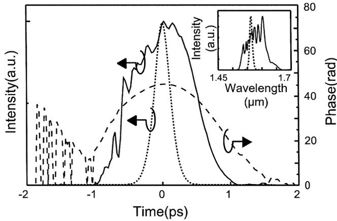
Fig. 2. Temporal and spectral waveform (solid line) and phase (broken line) of the pulses after propagation of normal dispersive EDF. Dotted line represents incident pulses.
