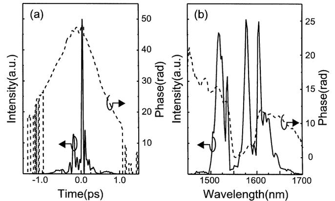
Fig. 4. Reconstructed (a) temporal waveform and (b) optical spectrum of generated high peak power femtosecond pulses.
