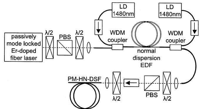
Fig. 1. Experimental setup for generation of high-power femtosecond pulse and ultrabroad SC.
