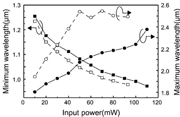
Fig. 6. Wavelength of the longest (circles) and the shortest (squares) wavelength edge of generated SC in 20-cm-long (filled data points and solid line) and 2-m-long (open data points and broken line) PM-HNL-DSFs as a function of the input average power.
