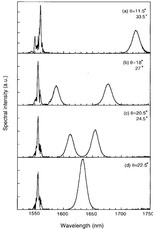
Fig. 2. Optical spectra of the output beam when  $\theta =$  (a)  $11.5^\circ$  and  $33.5^\circ$ , (b)  $18^\circ$  and  $27^\circ$ , (c)  $20.5^\circ$  and  $24.5^\circ$ , and (d)  $22.5^\circ$ . The fiber length is 110 m and the input power is 11.2 mW.
