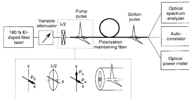
Fig. 1. Experimental setup of the proposed wavelength tunable two-colored fs soliton pulse generation.
