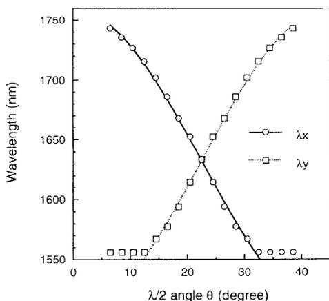
Fig. 4. Characteristics of wavelength shift in terms of the angle of the  $\lambda/2$  plate  $\theta$ . The fiber length is 110 m and the input power is 11.2 mW.
