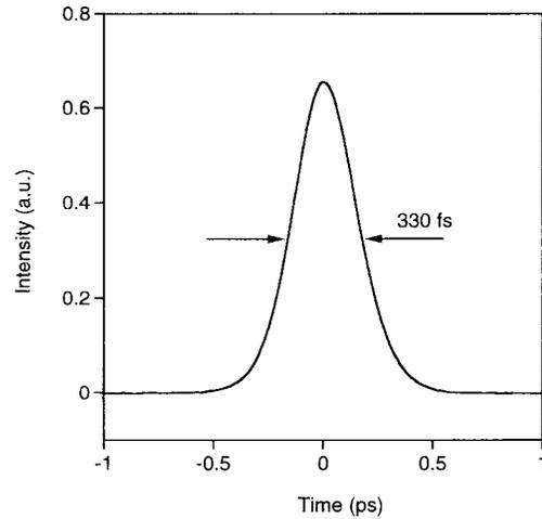
Fig. 3. Autocorrelation trace of horizontally polarized soliton pulse at 1652 nm when  $\theta = 20.5^\circ$ . The fiber length is 110 m and the input power is 11.2 mW.
