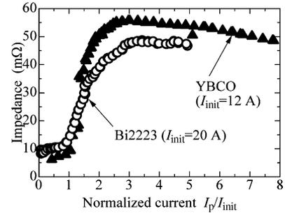
Fig. 6. Impedance of flat type FCL as a function of current.
