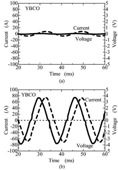
Fig. 5. Typical waveforms of current and voltage for YBCO version. (a)  $I_p = 7.45 A_{\text{peak}}$ ; (b)  $I_p = 71.5 A_{\text{peak}}$ .
