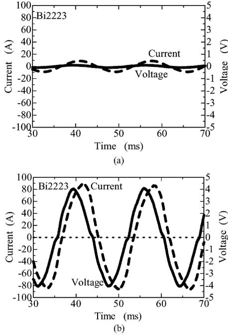
Fig. 4. Typical waveforms of current and voltage for Bi2223 version. (a)  $I_p = 8.85 A_{\text{peak}}$ ; (b)  $I_p = 84.7 A_{\text{peak}}$ .
