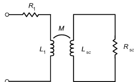
Fig. 2. Equivalent circuit of flat type fault current limiter.
