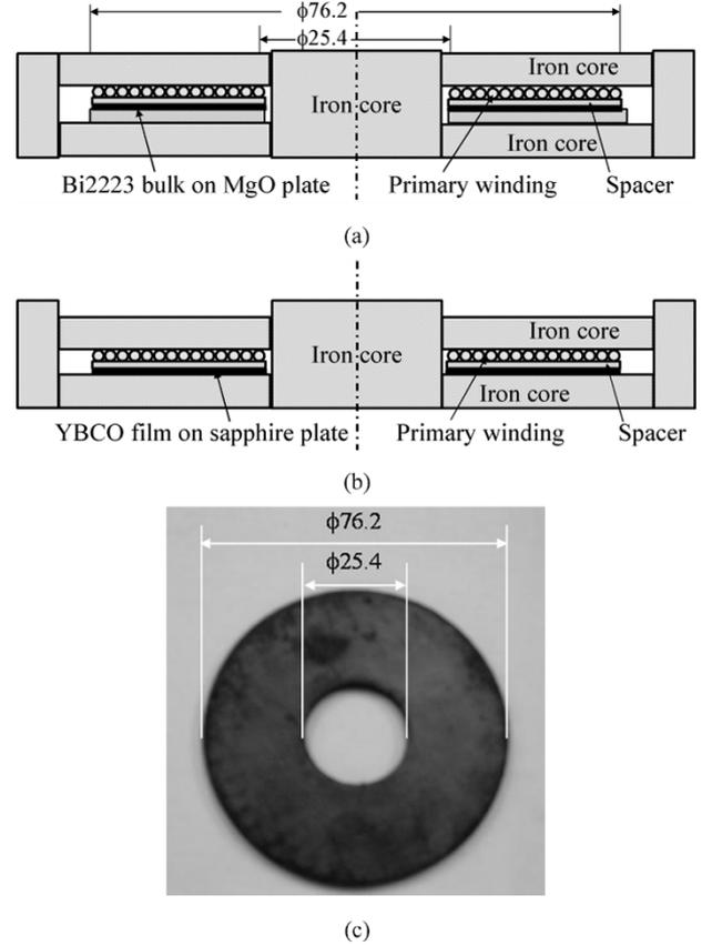
Fig. 3. Small models of flat type fault current limiter with HTS plate and iron core. (a) Small module of flat type FCL with Bi2223 bulk plate; (b) small module of flat type FCL with YBCO film plate; (c) Bi2223 bulk plate adopted.
