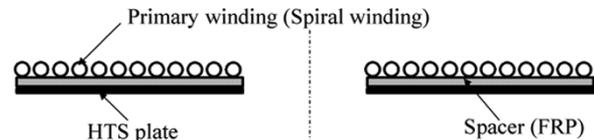
Fig. 1. Configuration of flat type of FCL.
