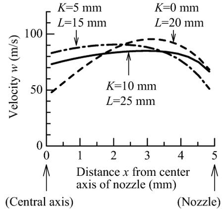
Fig. 5. Airflow velocity at a nozzle throat as a function of distance from central axis of nozzle for three cases. (Airflow rate:  $2.50 \times 10^{-3} \text{ m}^3/\text{s}$ , air temperature: 300 K).
