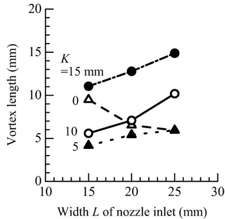
Fig. 8. Vortex length as a function of width  $L$  of nozzle inlet for different distances  $K$  between upstream electrode and nozzle inlet. (Airflow rate:  $2.50 \times 10^{-3} \text{ m}^3/\text{s}$ , air temperature: 300 K).
