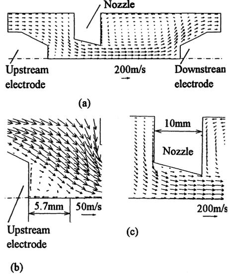
Fig. 4. Airflow velocity vectors calculated for distance  $K = 10$  mm from upstream electrode to nozzle throat and width  $L = 15$  mm of nozzle inlet under conditions of airflow rate of  $2.50 \times 10^{-3} \text{ m}^3/\text{s}$  and air temperature of 300 K.
