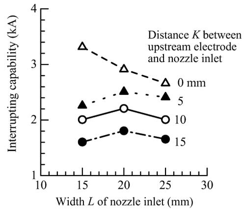
Fig. 3. Interrupting capability as a function of width  $L$  of nozzle inlet for different distances  $K$  between upstream electrode and nozzle inlet.
