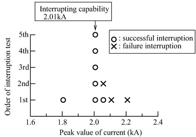
Fig. 2. Result of interruption test for distance  $K = 10$  mm between upstream electrode and nozzle throat and width  $L = 15$  mm of nozzle inlet.
