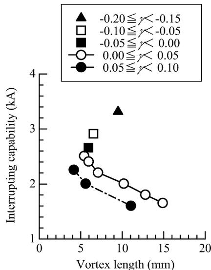
Fig. 9. Interrupting capability measured by interruption test as a function of vortex length determined by airflow-velocity calculation.
