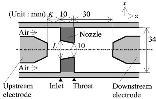
Fig. 1. Flat-type air-blast quenching chamber of 3 mm in thickness. This quenching chamber is sandwiched between two plates made of PTFE.
