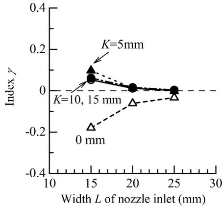
Fig. 6. Index  $\gamma$  of airflow-velocity profile at nozzle throat as a function of width  $L$  of nozzle inlet for different distances  $K$  between upstream electrode and nozzle inlet. (Airflow rate:  $2.50 \times 10^{-3} \text{ m}^3/\text{s}$ , air temperature: 300 K).
