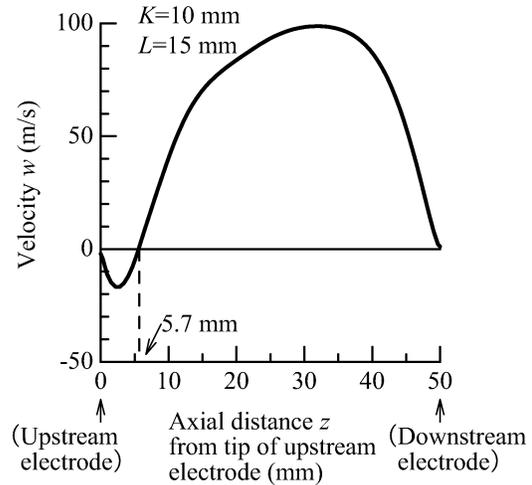
Fig. 7. Airflow velocity on central axis of quenching chamber as a function of axial distance from the tip of upstream electrode for  $K = 10$  mm and  $L = 15$  mm. (Airflow rate:  $2.50 \times 10^{-3} \text{ m}^3/\text{s}$ , Air temperature: 300 K).
