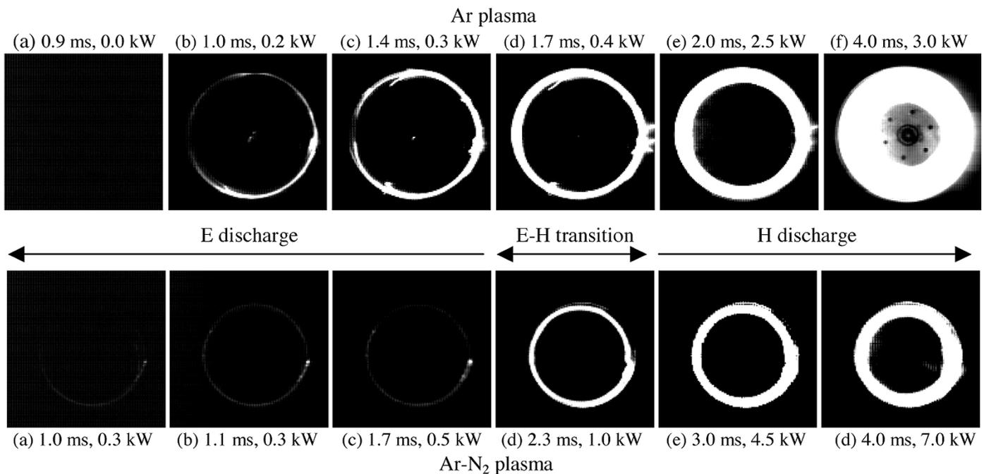
Fig. 2. Comparison of  $E$ - $H$  mode transition dynamics between pure Ar and Ar-N<sub>2</sub> plasmas with 10% N<sub>2</sub> in a pressure of 50 kPa.
