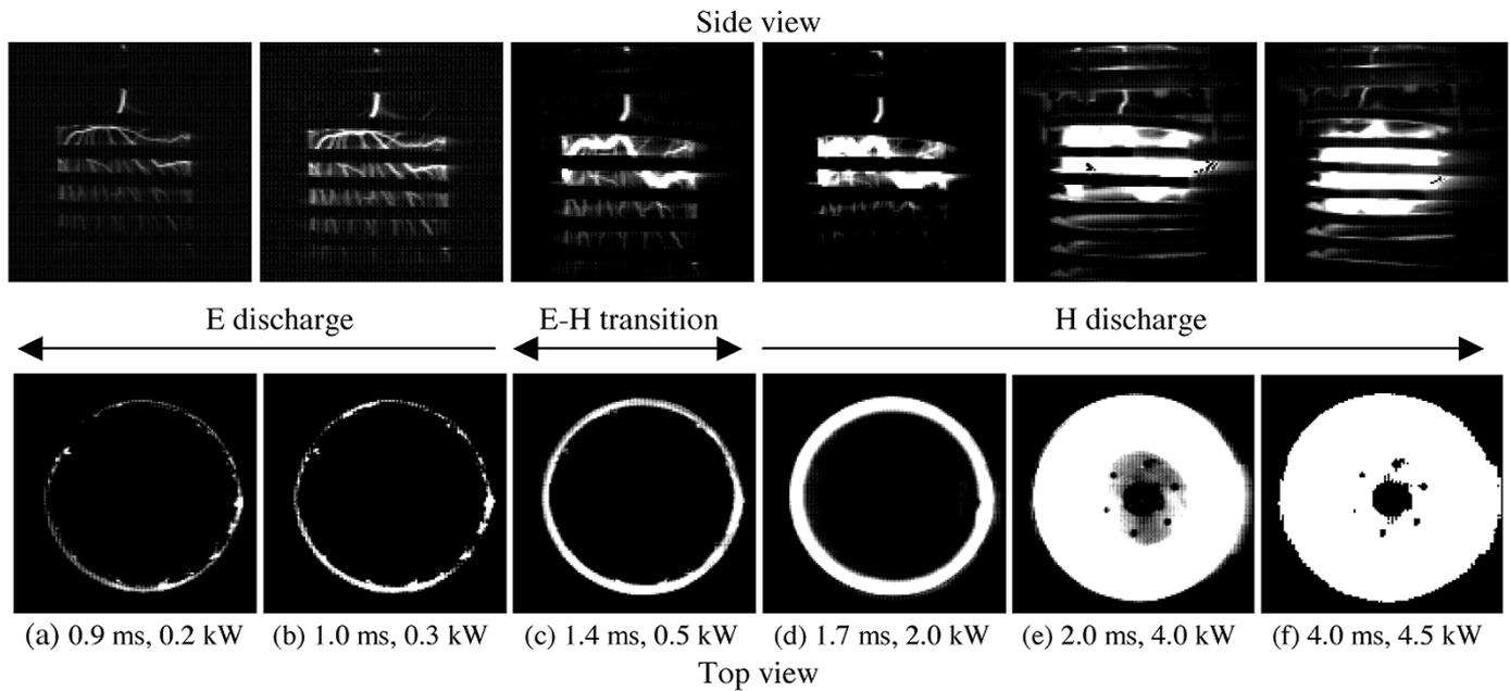
Fig. 1. Observation of  $E$ - $H$  mode transition in atmospheric pressure argon plasma. Timing and corresponding RF power are indicated below the respective image.
