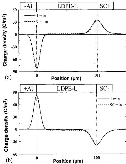
Figure 6. Space charge distribution in LDPE-L for (a) positive polarity and (b) negative polarity (applied field 50 MV/m, 40°C).
