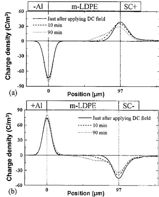
Figure 12. Space charge distribution in m-LDPE for (a) positive polarity and (b) negative polarity, under a dc field of 50 MV/m (23°C).
