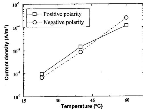
Figure 8. Temperature dependence of dc current (90 min) in LDPE-L under the application of a dc field of 50 MV/m.
