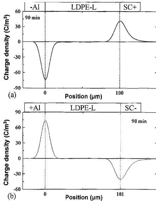
Figure 7. Space charge distribution in LDPE-L for (a) positive polarity and (b) negative polarity (applied field 50 MV/m, 60°C).
