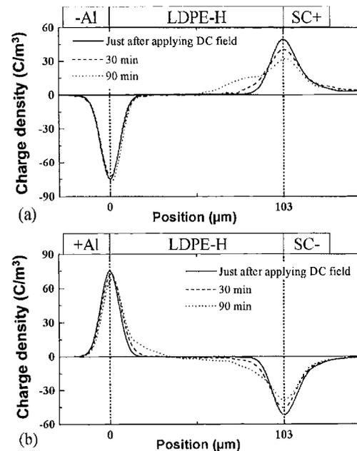
Figure 1. Space charge distributions in LDPE-H for (a) positive polarity and (b) negative polarity (applied field 50 MV/m, 23°C).
