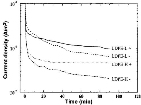
Figure 3. Current density vs. time characteristics (applied field: 50 MV/m, 23°C).
