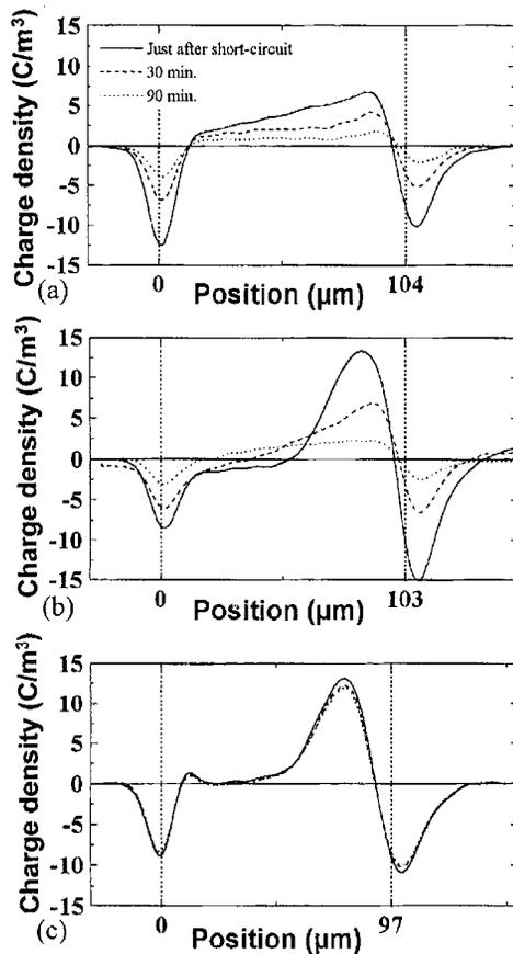
Figure 13. Space charge distribution in (a) LDPE-L, (b) LDPE-H and (c) m-LDPE after short-circuiting. A dc field of 50 MV/m was applied to the specimen for 90 min (23°C) and space charge was measured after short-circuiting.
