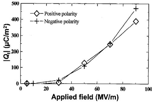
Figure 10. Total amount of space charge  $|Q_t|$  in the specimen, calculated from Figure 9.
