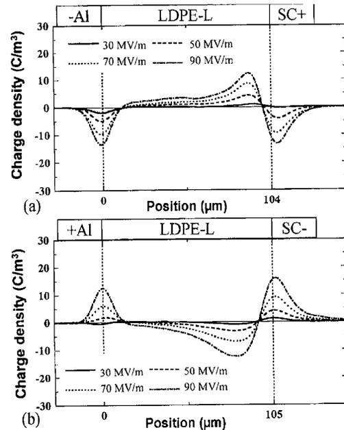
Figure 9. Space charge distribution in LDPE-L. Each dc field was applied for 10 min (23°C) and then space charge was measured just after short-circuiting.
