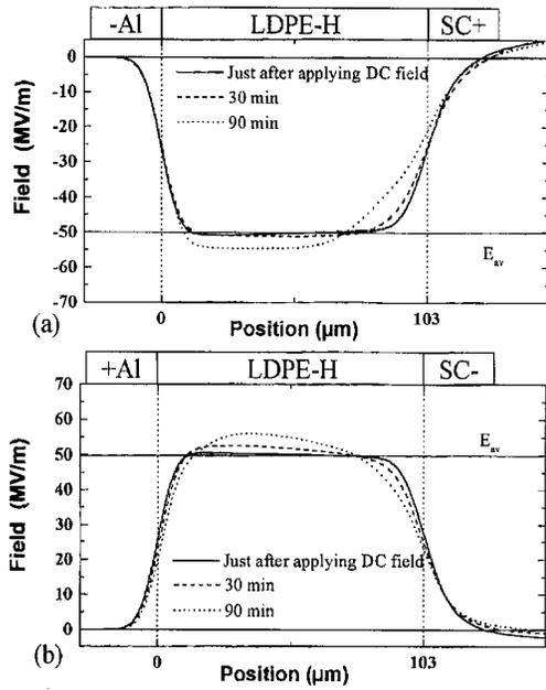
Figure 4. Field distribution in LDPE-H for (a) positive polarity and (b) negative polarity (applied field 50 MV/m, 23°C). Calculated from Figure 1.
