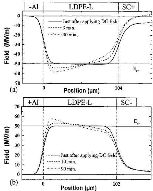
Figure 5. Field distribution in LDPE-L for (a) positive polarity and (b) negative polarity (applied field 50 MV/m, 23°C). Calculated from Figure 2.
