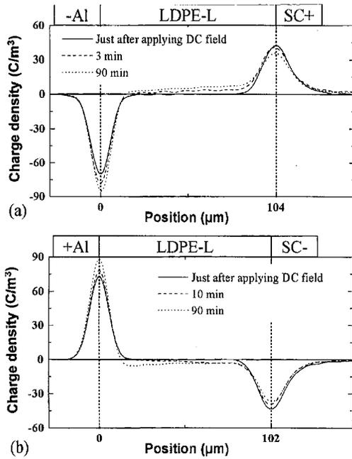
Figure 2. Space charge distributions in LDPE-L for (a) positive polarity and (b) negative polarity (applied field 50 MV/m, 23°C).
