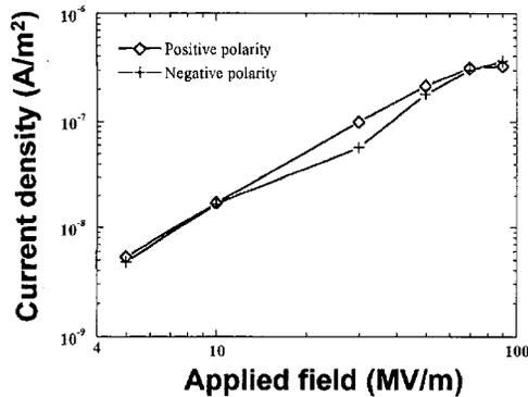
Figure 11. Current density measured 10 min after the application of dc field (23°C).
