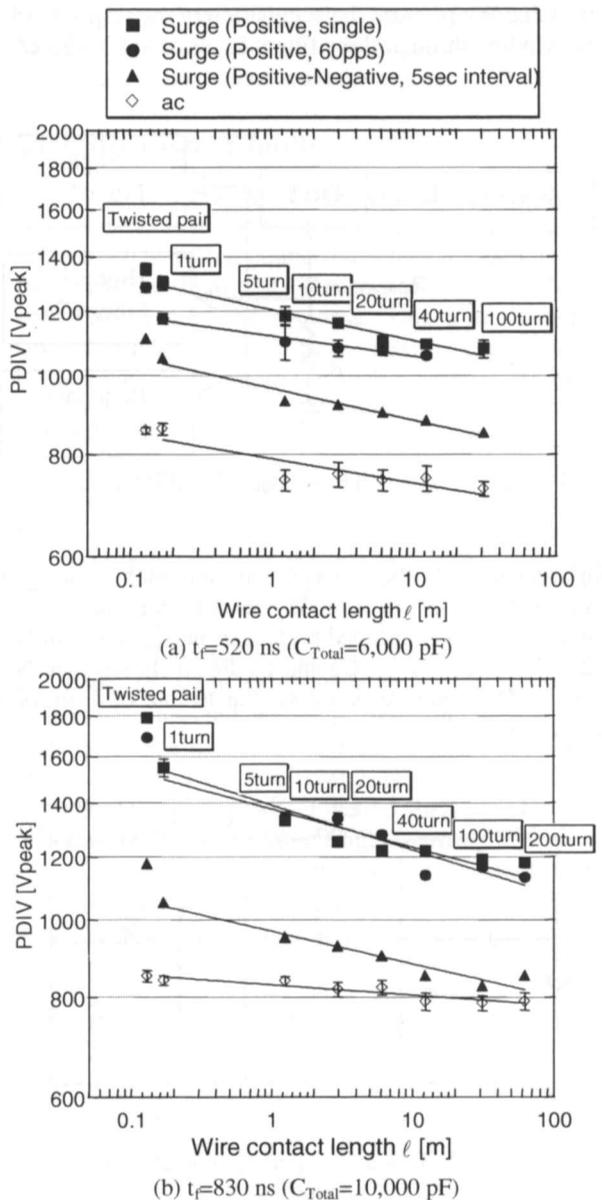
Figure 7: PDIV as a function of wire contact length
