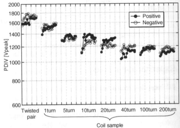
**Figure 6:** Surge PDIV for different test samples ( $t_f=520$  ns, 60 pps)
