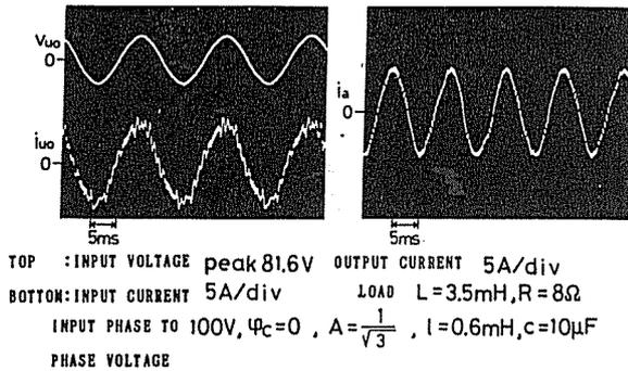
Fig. 14. Current waveforms at the input and the output (input 60Hz, output 90Hz,  $\varphi_s=0$ ).
