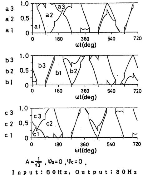
Fig. 11. Patterns of control functions  $a_1 \sim c_3$ .
