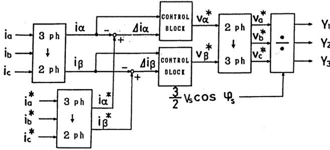
Fig. 10. Configuration of the output current control system.
