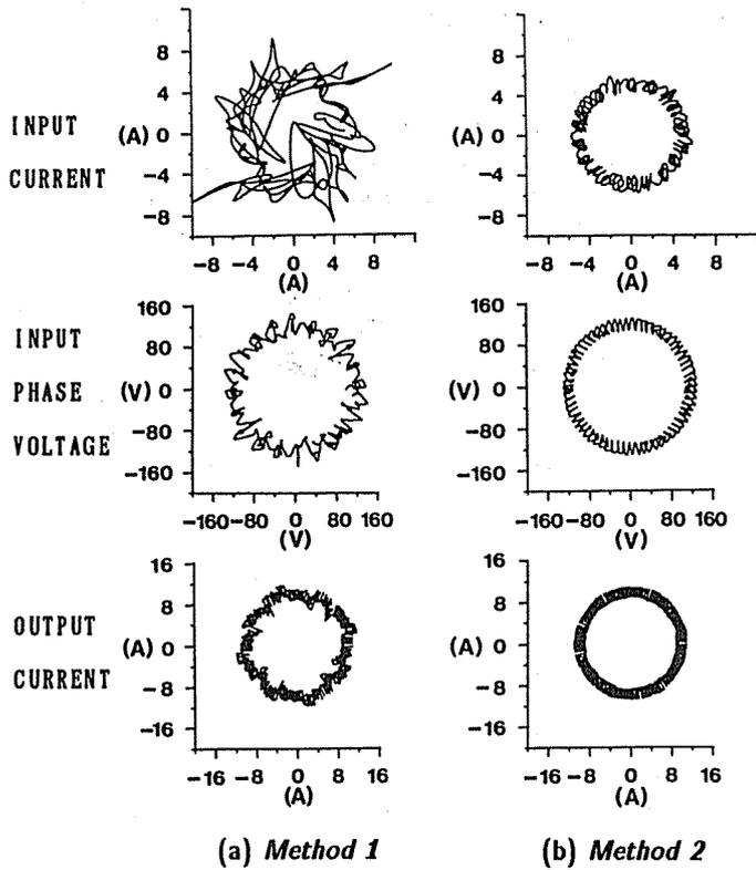
Fig. 17. Simulation results of *Method 1* and *Method 2*.
