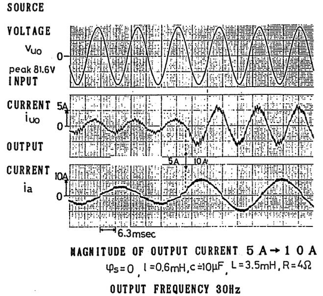
Fig. 19. Waveforms of the input and output current (with change of magnitude).
