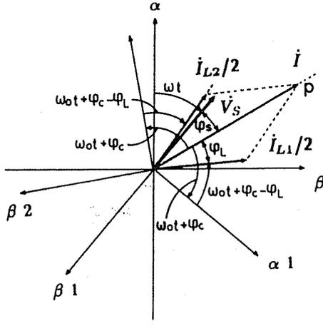
Fig. 4. Composition of input current vectors.
