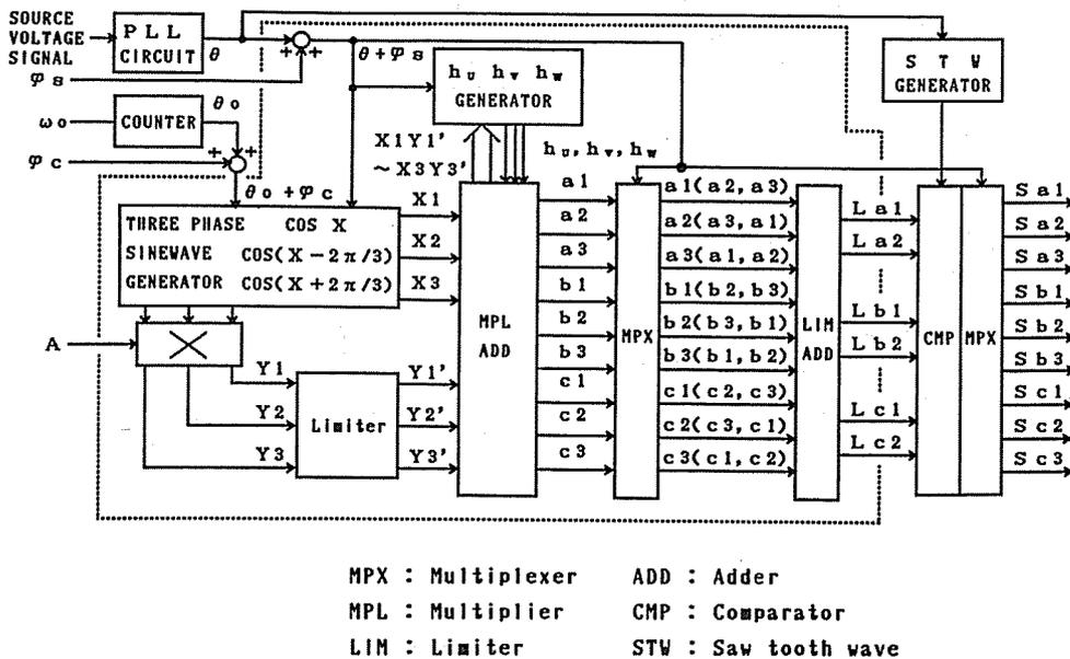
Fig. 9. System configuration.
