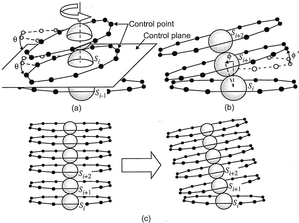
Figure 2. Rotational operation of vertebra spheres and control points.
