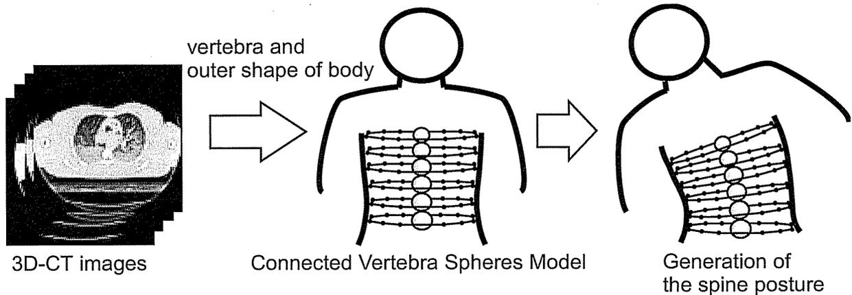
Figure 1. Concept of the spine posture estimation model.
