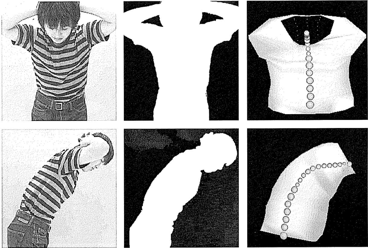
Figure 6. Experimental result to estimating forward bending. Left side column shows a couple of the input images. Center column shows silhouette images corresponding the left side column, Right side column shows the estimation results. This image displays by overlapping a spine posture on the image of the model's outer shape.
