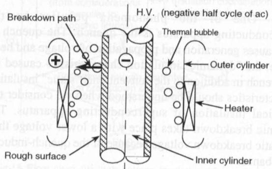
Fig.9 Schematic illustration of breakdown under combined conditions of rough surface electrode and thermal bubbles.
