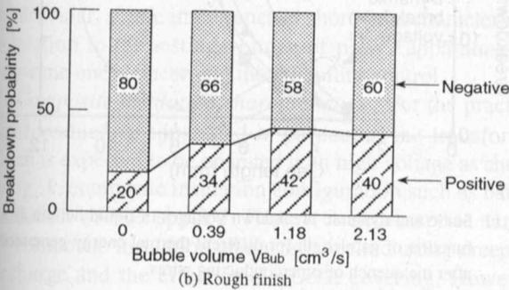
Fig.6 Breakdown probability at positive or negative half cycle of applied ac voltage for different bubble volume  $V_{Bub}$ .
