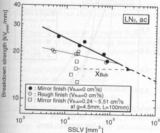
Fig.7 Breakdown strength as a function of SSLV with and without thermal bubble.
