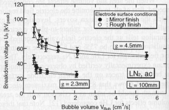
Fig.5 Breakdown voltage  $U_b$  as a function of bubble volume  $V_{Bub}$  for different electrode surface conditions and gap lengths.
