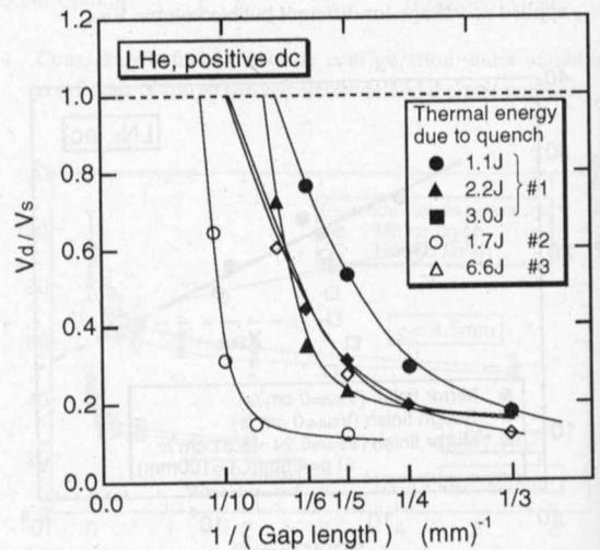
Fig.12 Reduction of breakdown voltage (*V<sub>d</sub>/V<sub>s</sub>*) as a function of (1/gap length) for different thermal energy generated after the quench of superconducting wires.
