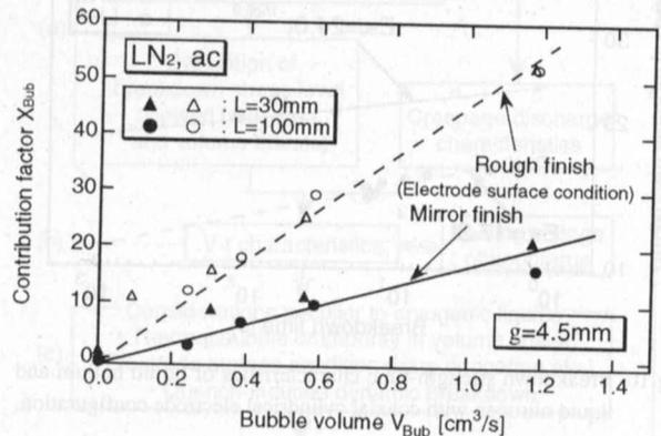
Fig.8 Contribution factor  $X_{Bub}$  of thermal bubbles as a function of bubble volume  $V_{Bub}$ .
