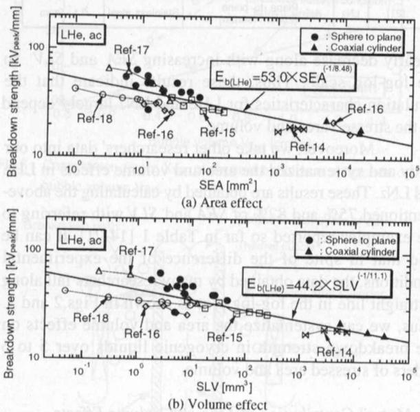
Fig.2 ac breakdown strength in liquid helium as a function of SEA and SLV (●,▲ : data by the authors; ○,△,□,◇,× : data by Table1).
