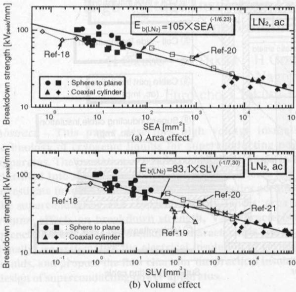
Fig.3 ac breakdown strength in liquid nitrogen as a function of SEA and SLV (●, ■, ▲, ◆ : data by the authors; △, □, ◇, ✕ : data by Table1).
