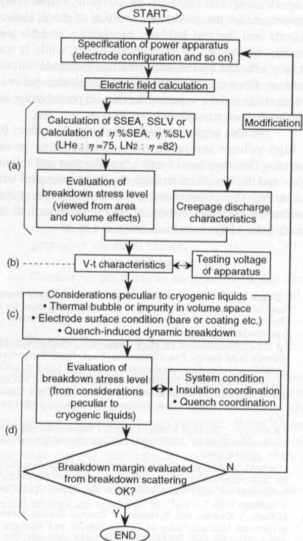
Fig.13 Flow chart for high voltage insulation of superconducting apparatus by cryogenic liquids.
