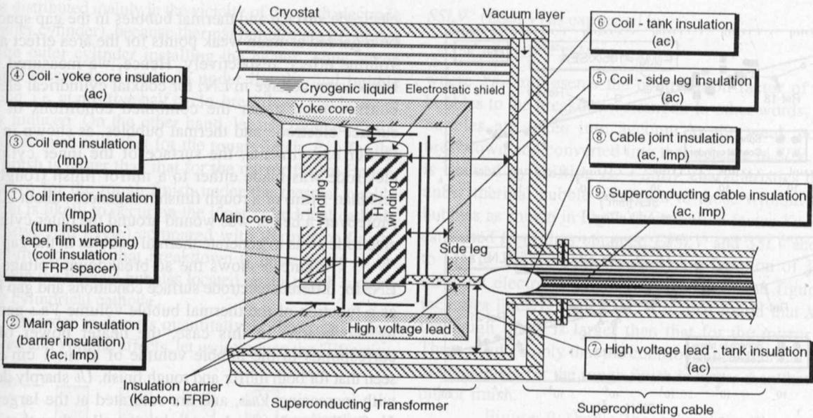
Fig.1 Classification of insulation component for pool cooling superconducting transformer and cable.
