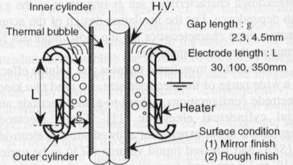
Fig.4 Coaxial cylindrical electrode configuration under combined conditions of rough surface electrode and thermal bubbles.
