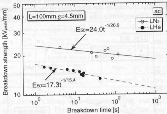
Fig.10 Breakdown strength-time characteristics of liquid helium and liquid nitrogen with coaxial cylindrical electrode configuration.
