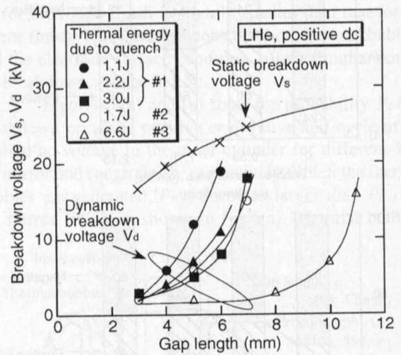
Fig.11 Static and dynamic breakdown voltages of liquid helium as a function of gap length for different thermal energy generated after the quench of superconducting wires.
