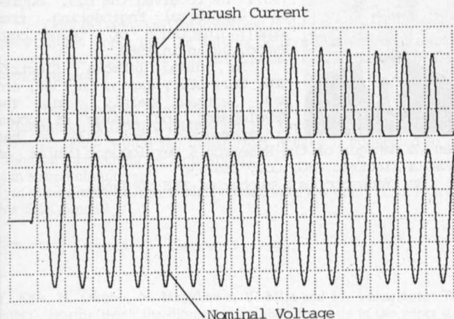
Fig. 10. Inrush current test: inrush current and the nominal voltage in the high-voltage winding (current : 8.3 A/div, voltage : 3700 V/div, time : 20 msec/div).
