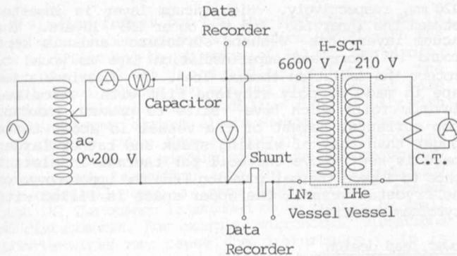
Fig. 7. A circuit diagram of the short-circuit test for the H-SCT.
