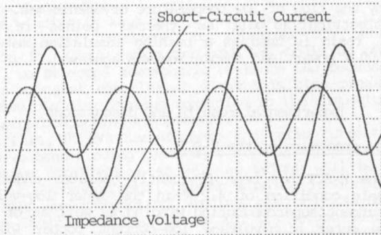
Fig. 8. Short-circuit test: short-circuit current and impedance voltage in the high-voltage winding (current : 8.3 A/div, voltage : 3000 V/div, time : 5 msec/div).
