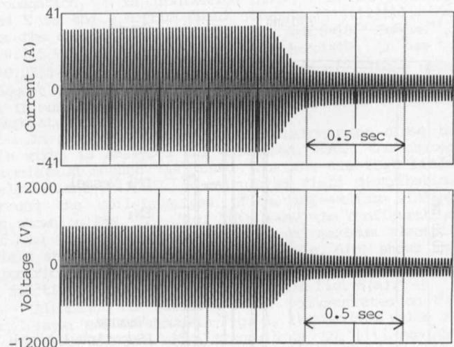
Fig. 9. Critical quenching current test: short-circuit current and the terminal voltage in the high-voltage winding.
