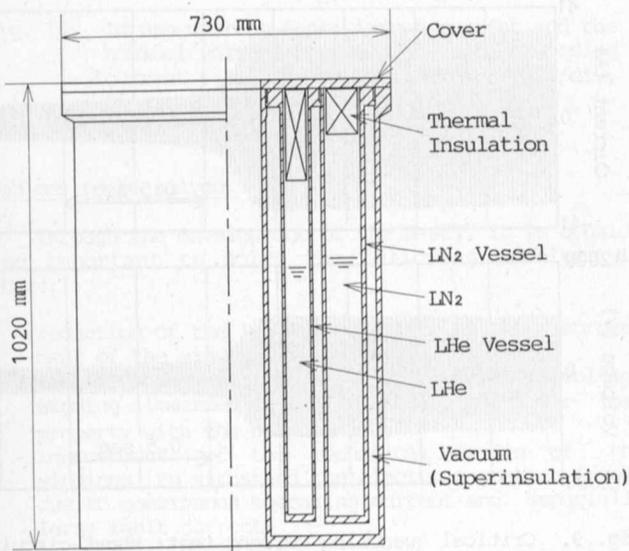
Fig. 6. Structure of the cryostat vessel.
