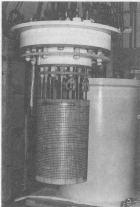
Fig. 4. Photograph of the superconducting low-voltage winding.
