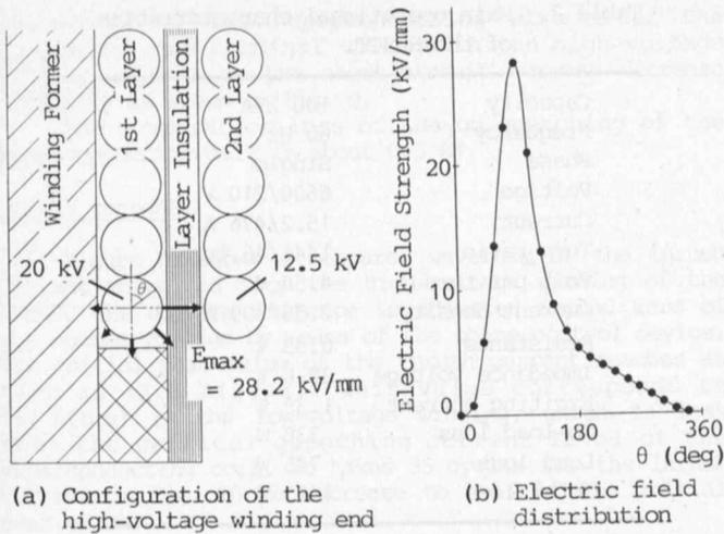
Fig. 5. Electric field distribution around the coil-layer end of the high-voltage winding.
