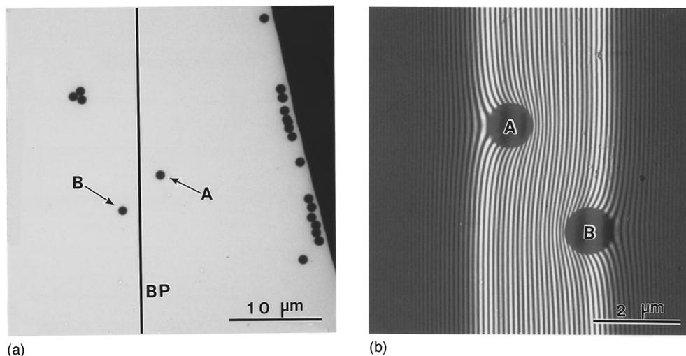
FIG. 3. (a) Low-magnified TEM image of polystyrene latex particles ( $d=1.0 \mu\text{m}$ ). (b) Two spheres indicated with arrow heads were recorded in an electron hologram from both sides of an electron biprism (BP).
