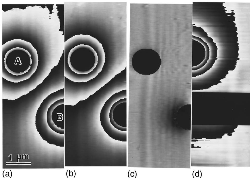
FIG. 4. Differential interferometry of latex spheres. (a) A phase image reconstructed from a hologram taken with the biprism potential  $V_{bp} = -13.0$  V; (b) another phase image of  $V_{bp} = -13.5$  V; (c) a one-dimensional differential image; and (d) integrated image showing a true phase distribution.
