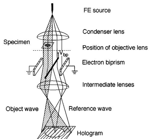
FIG. 1. Schematic electron-optical system for electron holographic interferometry.
