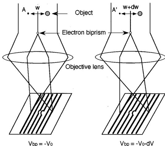
FIG. 2. Reference point overlapped with an object is sheared  $dw$  from A to A' by increasing the potential applied to an electron biprism  $-V_0$  to  $-V_0 - dV$ .
