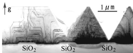
FIG. 3. Cross-sectional TEM image of an ELO-GaN structure on the  $[\bar{1}\bar{1}0]$ -oriented stripe-patterned Si substrate. The blurred image of the center triangle is due to local bending. Glue used in the TEM sample preparation process accidentally remained in the valley or pit region.  $g = 0002$ .
