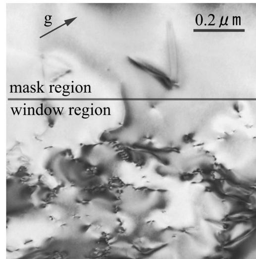
FIG. 2. Plan-view TEM image of a near-interface region of an ELO-GaN structure on the  $[11\bar{2}]$ -oriented stripe-patterned Si substrate. Both window and mask regions are imaged.  $\mathbf{g} = 11\bar{2}0$ .
