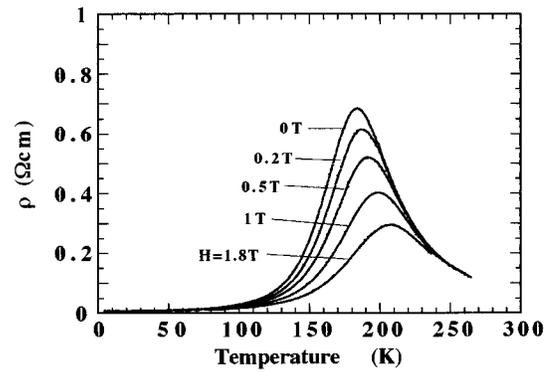
FIG. 2. Temperature dependence of resistivity  $\rho$  for a thin film of  $\text{La}_{3-3x}\text{Ca}_{1+3x}\text{Mn}_3\text{O}_{10}$  ( $x=0.3$ ) under various magnetic fields.
