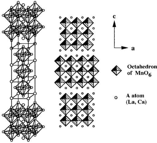
FIG. 1. Crystal structure and layer sequence of triple perovskite  $\text{La}_{3-3x}\text{Ca}_{1+3x}\text{Mn}_3\text{O}_{10}$ .
