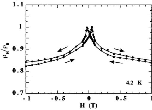
FIG. 4. Normalized resistivity  $\rho_H/\rho_0$  and magnetization as a function of applied magnetic field at 4.2 K for a thin film of  $\text{La}_{3-3x}\text{Ca}_{1+3x}\text{Mn}_3\text{O}_{10}$  ( $x=0.3$ ). These data were obtained after an initial application of a magnetic field of +1.8 T, and sampling cycles are shown as arrows. The solid lines are drawn only as a guide to the eyes.
