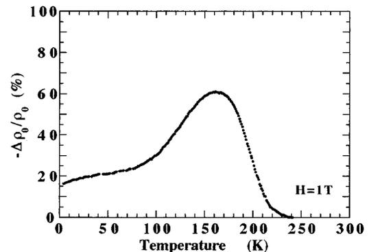
FIG. 3. Temperature dependence of the MR ratio ( $-\Delta\rho/\rho_0$ ) in  $H=1$  T for a thin film of  $\text{La}_{3-3x}\text{Ca}_{1+3x}\text{Mn}_3\text{O}_{10}$  ( $x=0.3$ ). The MR ratio is calculated from the data in Fig. 2.
