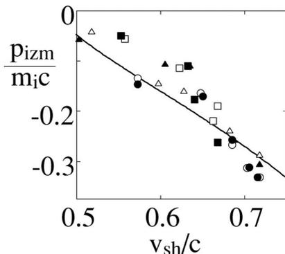
FIG. 7. Ion momentum  $p_{iz}$  at  $x=x_m$ ,  $p_{izm}$ , versus shock speed  $v_{sh}$ . The closed and open symbols refer to the results with  $v_{Te}=0.4$  and  $v_{Te}=1.5$ , respectively. The circles, triangles, and squares show measurements at  $\omega_{pe}t=300$ , 600, and 900, respectively.
