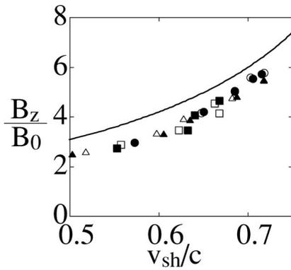
FIG. 6. The maximum value of  $B_z$  versus shock speed  $v_{sh}$ . The solid line shows the theory. The closed and open symbols denote simulation results with  $v_{Te}=0.4$  and  $v_{Te}=1.5$ , respectively. The circles, triangles, and squares show values averaged over time from  $\omega_{pe}t=0$  to  $\omega_{pe}t=300$ , from 300 to 600, and from 600 to 900, respectively.
