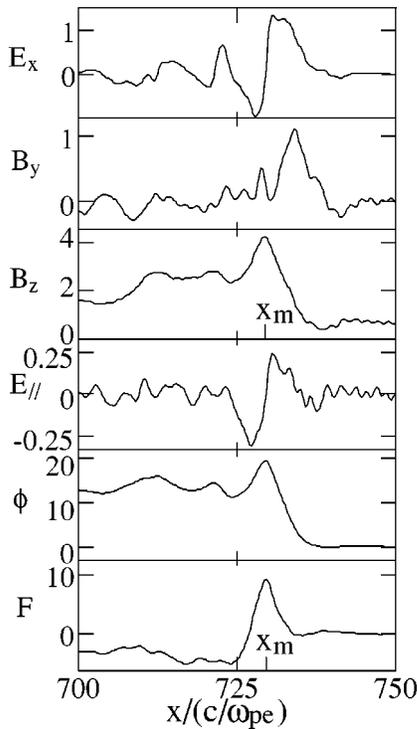
FIG. 3. Snapshots of field profiles at  $\omega_{pe}t=900$ . Electric and magnetic fields are normalized to  $B_0$ , while  $\phi$  and  $F$  are normalized to  $m_e c^2/e$ . The quantities  $B_z$ ,  $\phi$ , and  $F$  take their maximum values at  $x=x_m$ .
