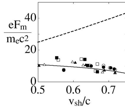
FIG. 8. The maximum value of  $F$  versus shock speed  $v_{sh}$ . The solid line shows the theory. The closed and open symbols denote simulation results with  $v_{Te}=0.4$  and  $v_{Te}=1.5$ , respectively. The circles, triangles, and squares show values averaged over time from  $\omega_{pe}t=0$  to  $\omega_{pe}t=300$ , from 300 to 600, and from 600 to 900, respectively.
