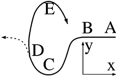
FIG. 2. Schematic diagram of electron guiding-center orbits in the  $(x, y)$  plane in the wave frame. Point A is in the upstream region. The  $x$  positions of points C and E are  $x = x_m$ . Passing electrons move as  $A \rightarrow B \rightarrow C \rightarrow D$ —dashed line. Some electrons can be reflected at point D and then trapped.
