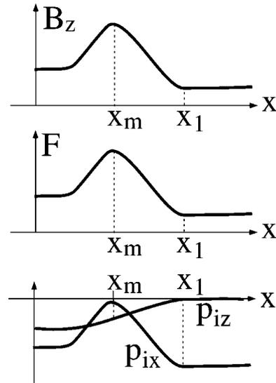
FIG. 1. Schematic diagram of  $B_z$ ,  $F$ , and ion momenta  $p_{ix}$  and  $p_{iz}$  in the wave frame. The position  $x_l$  indicates the leading edge of the shock wave, and  $x_m$  is the point where  $B_z$  takes its maximum value.
