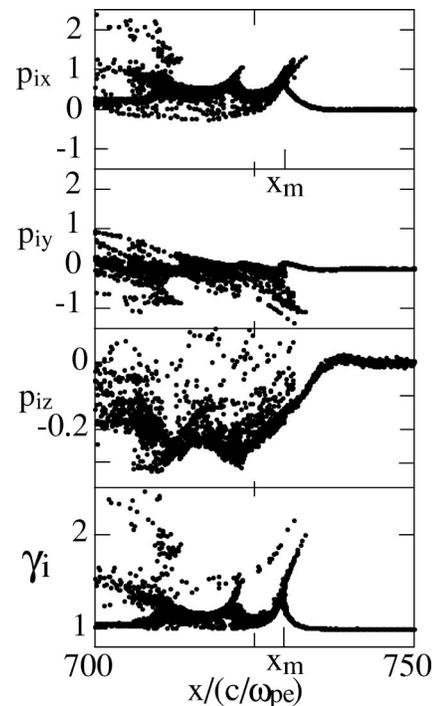
FIG. 5. Phase space plots of ions. The momenta are normalized to  $m_i c$ . As the ions penetrate the shock region,  $p_{iz}$  decreases.
