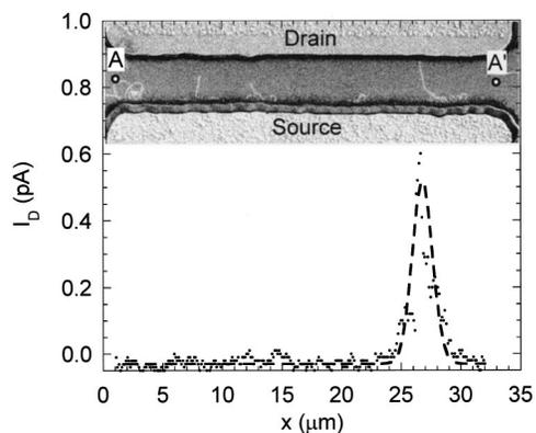
FIG. 2.  $\mu$ -PC as a function of position between  $A$  and  $A'$  shown in SEM image of the inset. The dotted line is a Gaussian fit.
