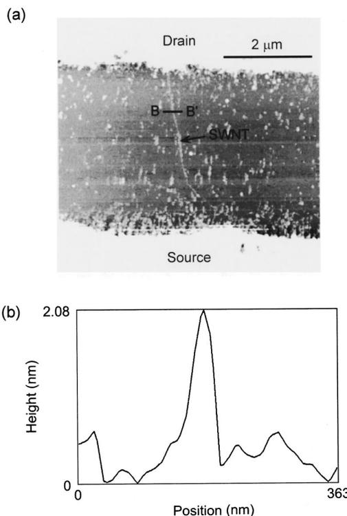
FIG. 3. (a) AFM image at the position where  $\mu$ -PC was observed in Fig. 2, and (b) cross-sectional profile between  $B$  and  $B'$ .
