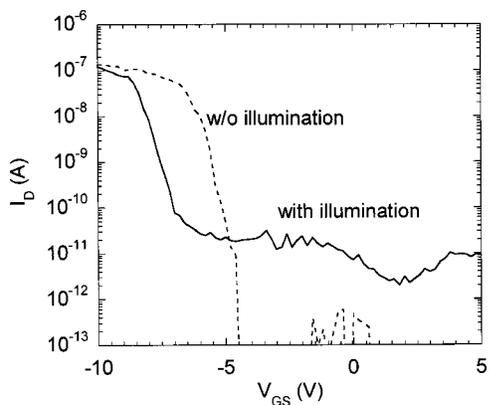
FIG. 1.  $I_D$ - $V_{GS}$  characteristics of nanotube FET in dark (dashed line) and under illumination (solid line).
