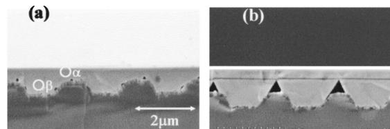
FIG. 1. Cross-sectional scanning electron micrograph image of the samples (a) without and (b) with an LT-ALN layer. The CL spectra shown in Fig. 2 are obtained at positions  $\alpha$  and  $\beta$ .
