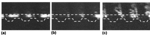
FIG. 3. Cross-sectional CL images for a sample shown in Fig. 1(a): (a) 358, (b) 363, and (c) 376 nm. The broken lines indicate the boundary of the GaN section.
