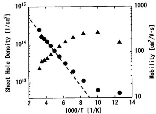
FIG. 4. Hole density ( $\bullet$ ) and mobility ( $\blacktriangle$ ) vs  $1/T$  for sample (A).
