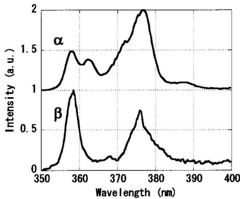
FIG. 2. CL spectra measured at 4.2 K. Top trace ( $\alpha$ ) is near the surface and bottom trace ( $\beta$ ) is on the stripe structure [see Fig. 1(a)]. The top trace has two subsidiary peaks at 363 nm and 372 nm.
