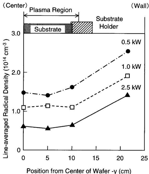
FIG. 2. Spatial distribution of absolute  $\text{CF}_2$  radical density as a function of microwave power.
