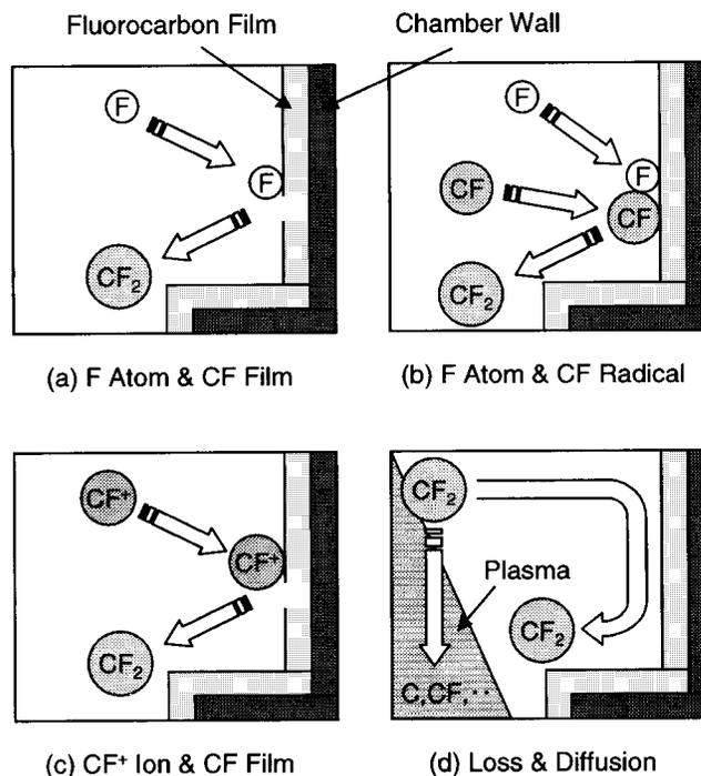
FIG. 3. Four models for formation of hollow  $\text{CF}_2$  radical distribution; (a) etching reaction between F atoms and fluorocarbon films, (b) three-body association between CF radicals and F atoms, (c) sputtering of fluorocarbon film by  $\text{CF}_x^+$  ions or neutralization of  $\text{CF}_x^+$  ions, and (d) intensive loss in plasma region and diffusion of  $\text{CF}_2$  radicals.
