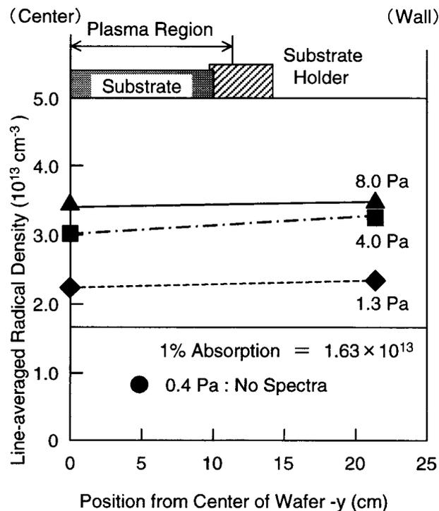
FIG. 10. Spatial distribution of the absolute  $\text{CF}_3$  radical density as a function of pressure.
