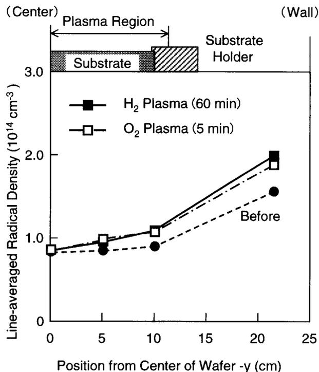
FIG. 4. Spatial distribution of the absolute  $CF_2$  radical density after  $H_2$  or  $O_2$  plasma pretreatment.
