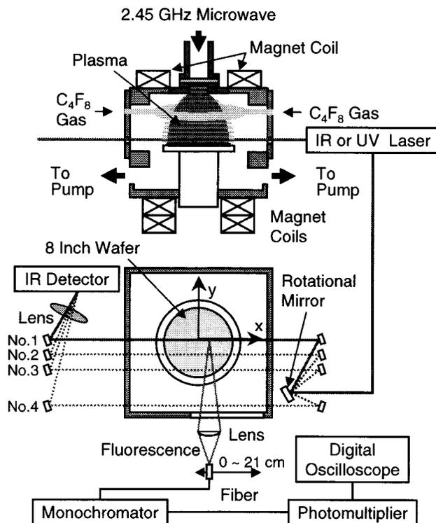
FIG. 1. Schematic diagram of ECR plasma reactor and radical measurement systems with single-pass IRLAS and LIF measurement systems.
