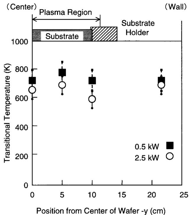
FIG. 5. Spatial distribution of the translational temperatures of  $CF_2$  radicals as a function of microwave power.
