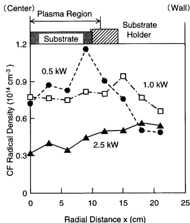
FIG. 8. Precise spatial distribution of the absolute CF radical density as a function of microwave power.
