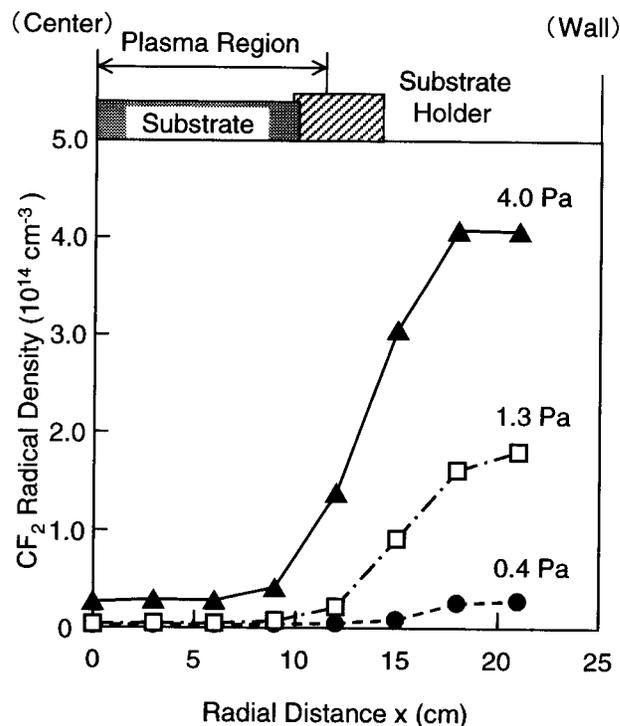
FIG. 7. Precise spatial distribution of the absolute  $CF_2$  radical density as a function of pressure.
