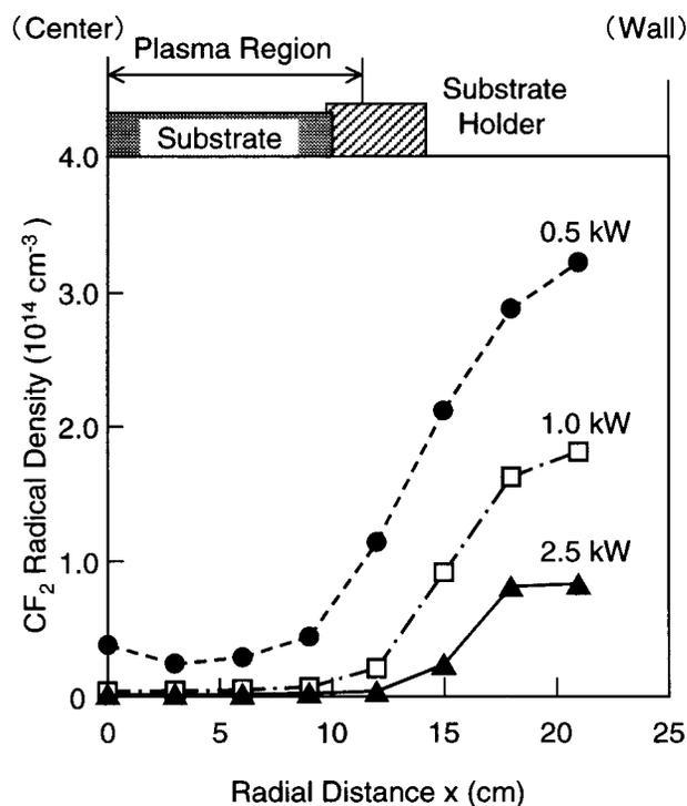
FIG. 6. Precise spatial distribution of the absolute  $CF_2$  radical density as a function of microwave power.
