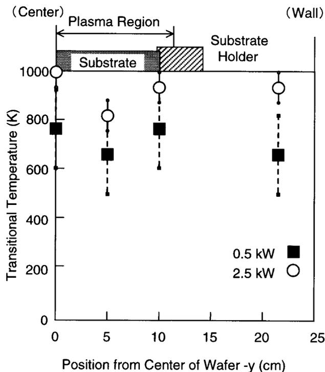
FIG. 9. Spatial distribution of the translational temperatures of CF radicals as a function of microwave power.
