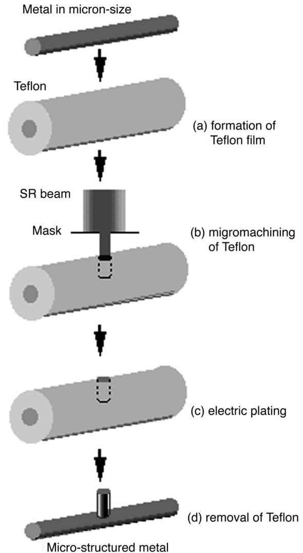
FIG. 14. Schematic diagram of the procedure for the fabrication of metal microparts using the SR ablation process. This procedure consists of (a) Teflon film formation on the curved surface of a metal substance in micron size using the SR ablation, (b) micromachining of Teflon film using the SR ablation, (c) electric plating, and (d) removal of Teflon film.
