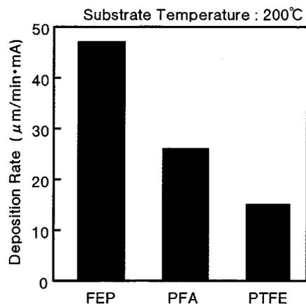
FIG. 11. Deposition rates of fluorocarbon films formed at a substrate temperature of 200 °C using SR ablation of PTFE, PFA, and FEP targets.
