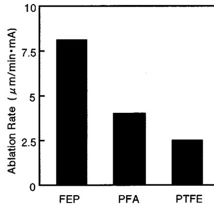
FIG. 7. Ablation rates of PTFE, PFA, and FEP in the case using a Ni mask with a 77  $\mu\text{m}$  square-hole pattern.
