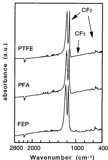
FIG. 12. FTIR spectra of films deposited using SR ablation of PTFE, PFA, and FEP at a dose of 50 min mA and a substrate temperature of 200 °C.
