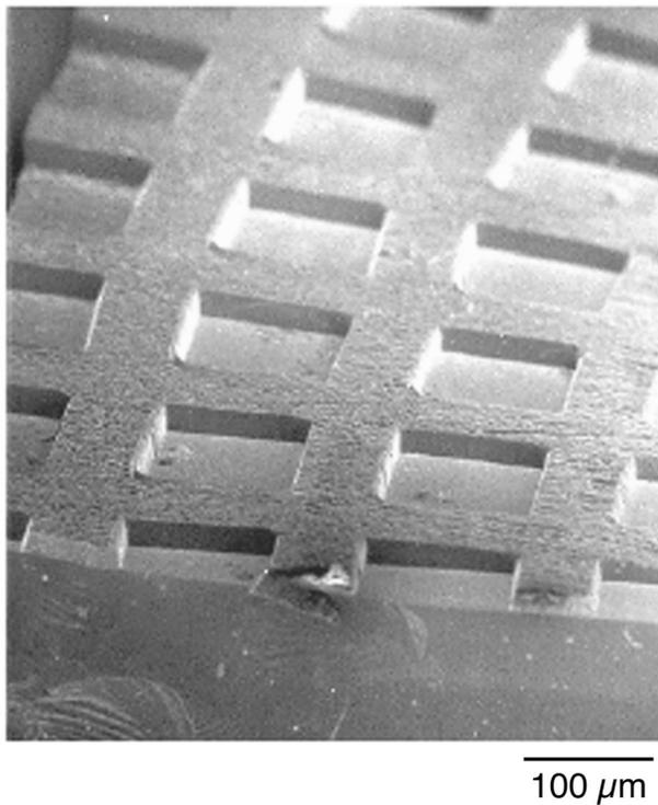
FIG. 13. SEM photograph of SR-ablated pattern created in Teflon film formed at a substrate temperature of 200 °C by SR ablation of FEP.
