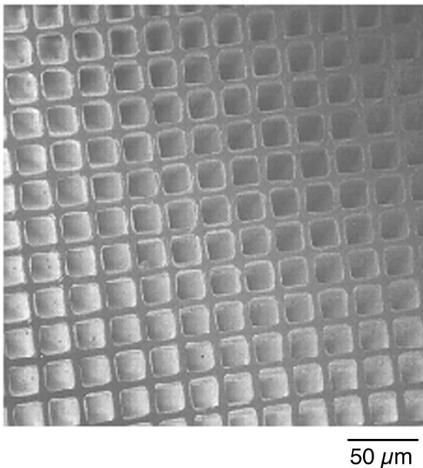
FIG. 5. SEM photograph of fine pattern with 19  $\mu\text{m}$  square holes created in FEP by the SR ablation process.
