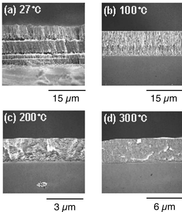
FIG. 8. Cross sectional SEM images of PTFE films formed at substrate temperatures of (a) 27 °C, (b) 100 °C, (c) 200 °C, and (d) 300 °C by the SR ablation process.
