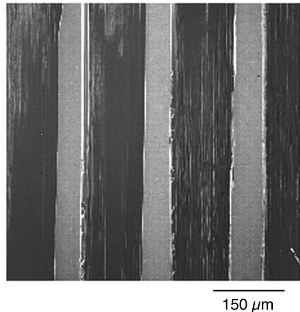
FIG. 4. Cross sectional SEM image of PTFE fine pattern with 77  $\mu\text{m}$  square holes created in PTFE created by the SR ablation process.
