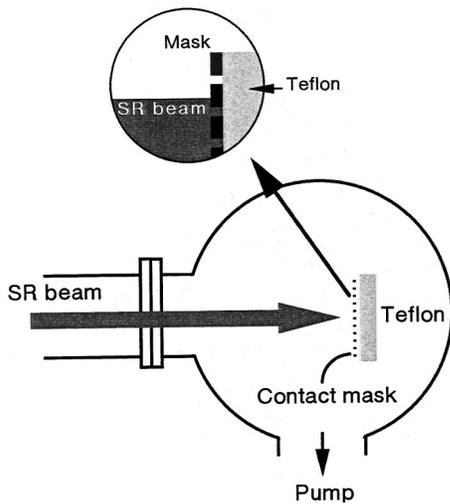
FIG. 1. Schematic diagram of experimental apparatus used to micromachining of Teflon by the SR ablation process.
