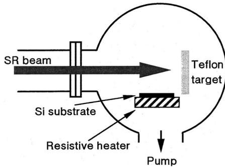
FIG. 2. Schematic diagram of experimental apparatus used for film formation of Teflon by the SR ablation process.
