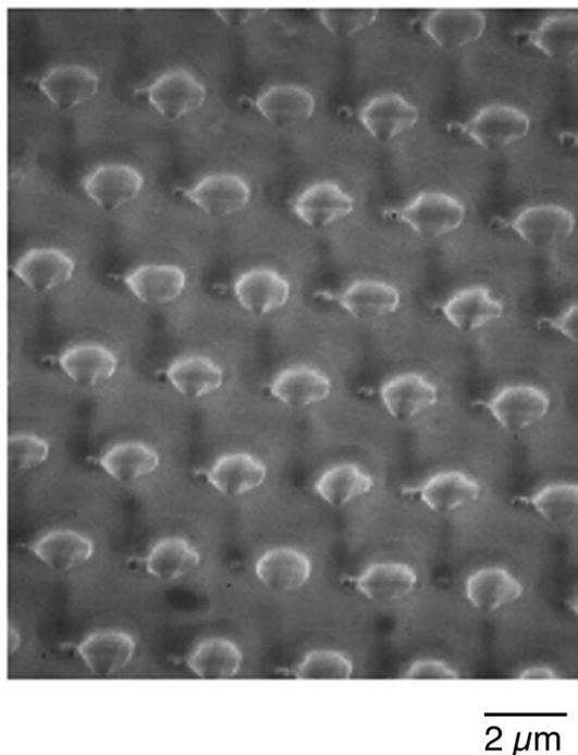
FIG. 6. SEM photograph of fine pattern with 2  $\mu\text{m}$  holes created in PTFE by the SR ablation process.
