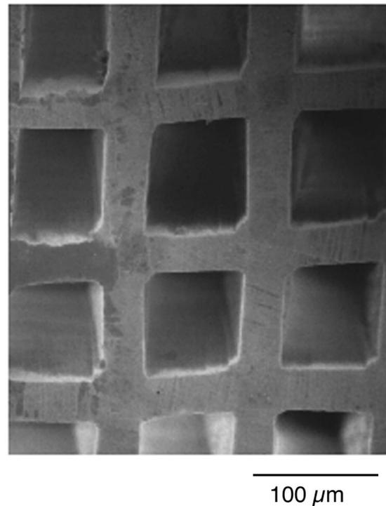
FIG. 3. SEM photograph of fine pattern with 77  $\mu\text{m}$  square holes created in PTFE by the SR ablation process.
