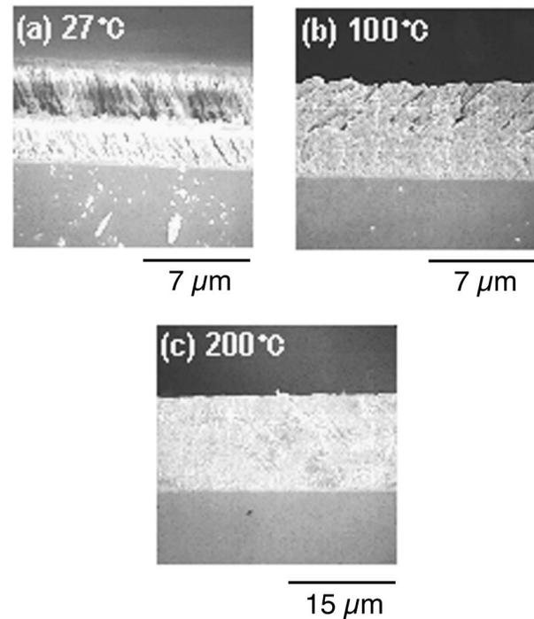
FIG. 10. Cross sectional SEM images of FEP films formed at substrate temperatures of (a) 27 °C, (b) 100 °C, and (c) 200 °C by the SR ablation process.
