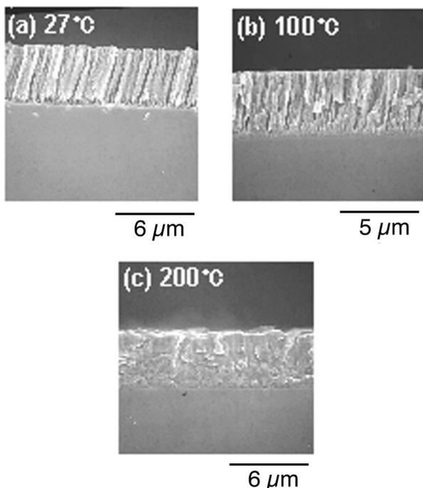
FIG. 9. Cross sectional SEM images of PFA films formed at substrate temperatures of (a) 27 °C, (b) 100 °C, and (c) 200 °C by the SR ablation process.
