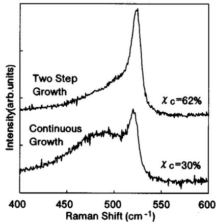
FIG. 3. Raman spectra of the films formed by two step growth (upper panel) and the continuous growth (lower panel).
