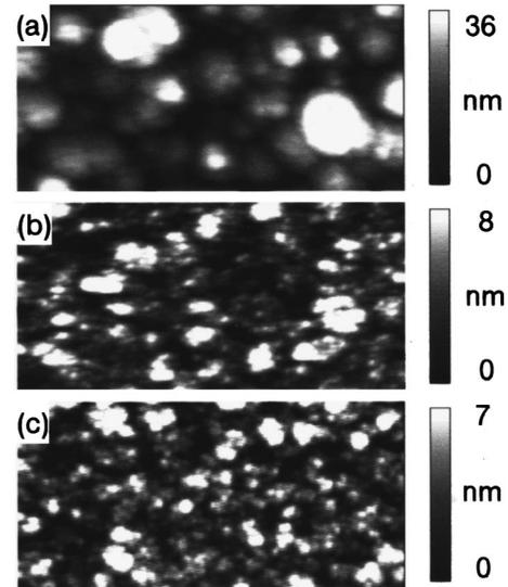
FIG. 2. AFM images ( $500\text{ nm} \times 1000\text{ nm}$ ) of the films formed (a) with and (b) without charged species and (c) by two step growth.
