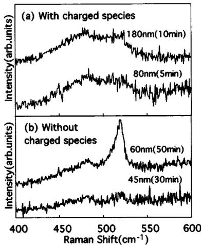
FIG. 1. Raman spectra for the poly-Si films formed (a) with and (b) without charged species in the initial growth.
