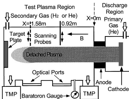
FIG. 2. Schematic of experimental apparatus NAGDIS-II. The running magnetic field strength is  $0.25$  T. The length of the plasma in the test plasma region is  $2$  m and the diameter of the vacuum vessel is  $0.19$  m.
