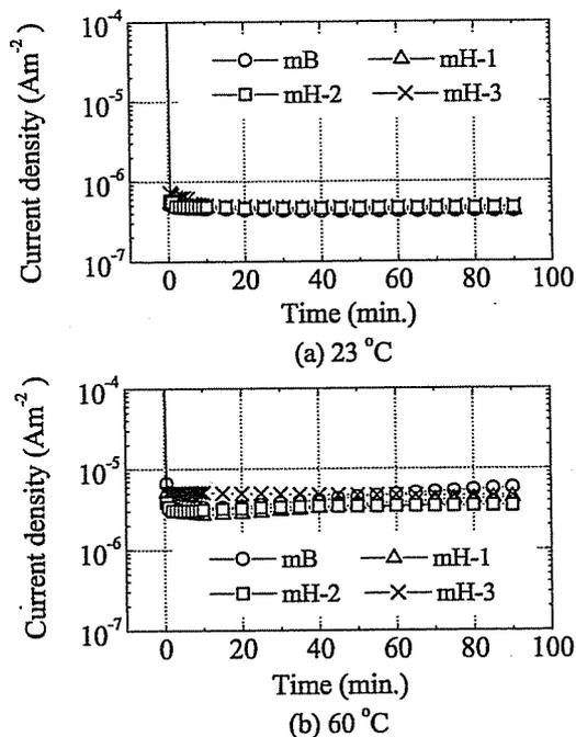
Fig. 7 DC charging current at 23 °C (a) and 60 °C (b) (50 MV/m)
