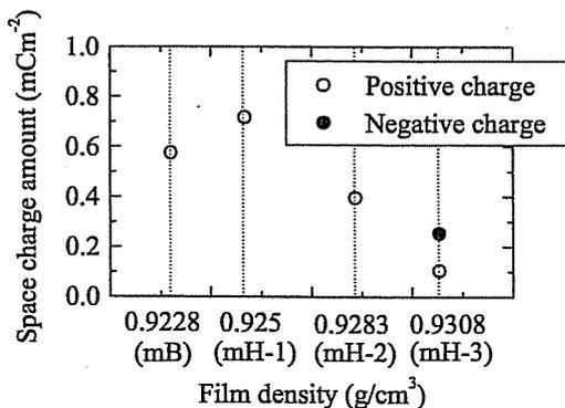
Fig. 6 Dependence of space charge amount on film density (50 MV/m, 60 °C)
