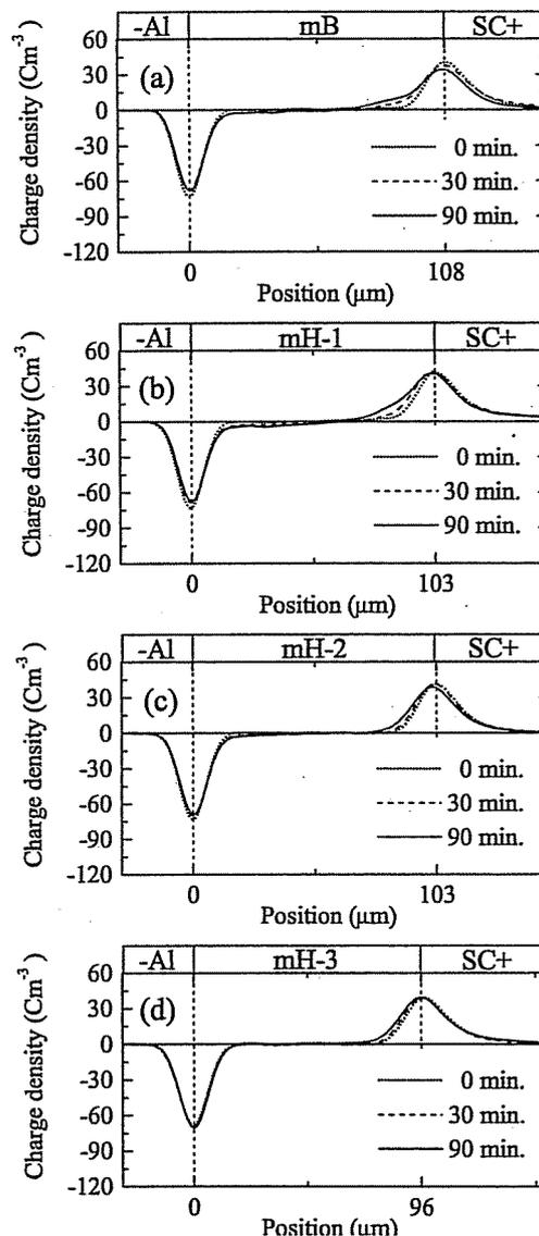
Fig. 3 Space charge distributions in mB (a), mH-1 (b), mH-2 (c) and mH-3 (d) at 23 °C (50 MV/m)
