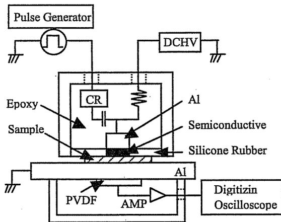
Fig. 1 Setup for space charge measurement (PEA method)
