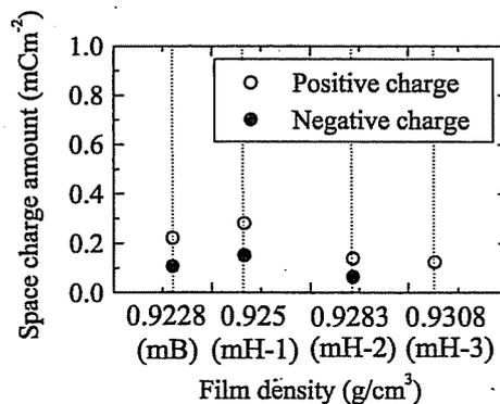
Fig. 4 Dependence of space charge amount on film density (50 MV/m, 23 °C)
