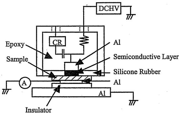
Fig. 2 Setup for DC current measurement
