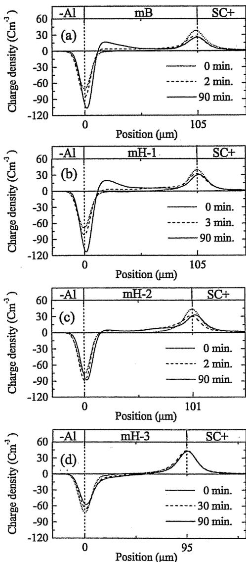
Fig. 5 Space charge distributions in mB (a), mH-1 (b), mH-2 (c) and mH-3 (d) at 60 °C (50 MV/m)
