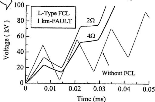
(b) Initial short-line-fault TRV for the L-Type FCL
