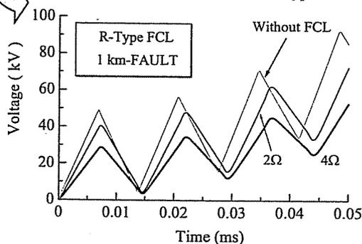
(b) Initial short-line-fault TRV for the R-Type FCL
