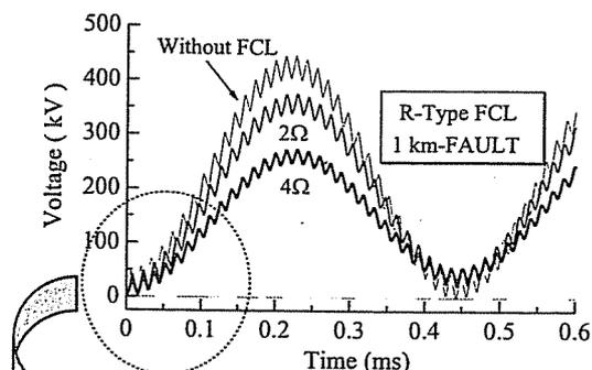
(a) Short-line-fault TRV for the R-Type FCL
