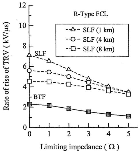
Figure 6. Rate of rise of the TRV as a function of the limiting impedance for the resistive FCL.
