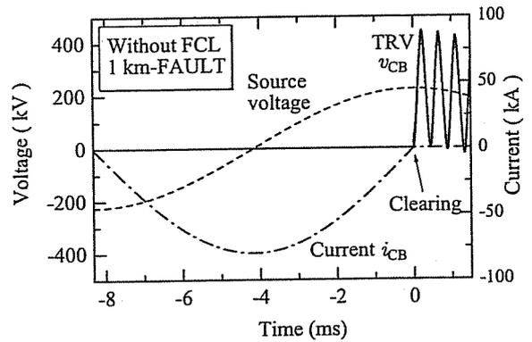
Figure 3. TRV following interruption of the fault current in the absence of the FCL.
