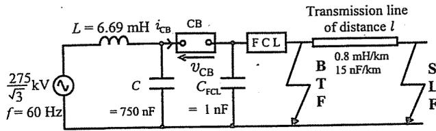
Figure 1. Single-phase equivalent circuit of a symmetrical three-phase-to-ground short circuit.
