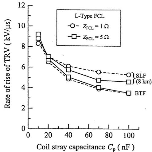
Figure 9. Dependence of the rrv on the stray capacitance of the limiting coil.
