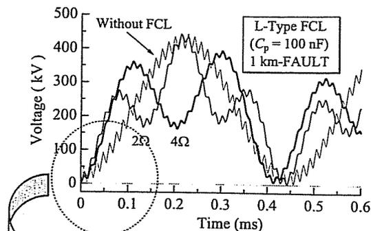
(a) Short-line-fault TRV for the L-Type FCL
