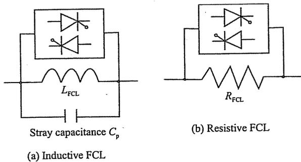
Figure 2. Equivalent circuit for each semiconductor type of FCL in current-limiting operation
