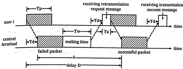
Fig. 1 Elapsed time between packets when the retransmission is required.
