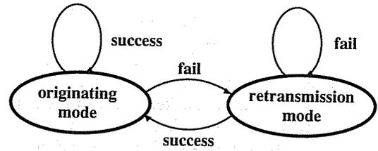
Fig. 2 Transition of users between the originating mode and the retransmission mode.
