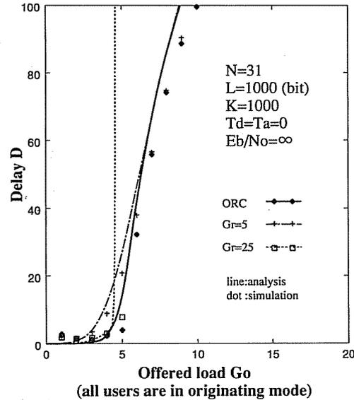
Fig. 6 Delay performance as a function of the offered load.
