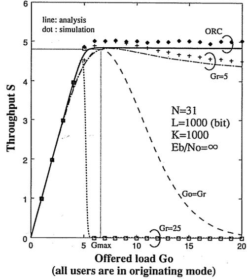
Fig. 5 Throughput performance as a function of the offered load.
