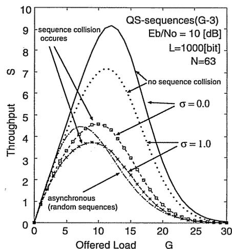
Fig. 9 Performance degradation due to the collision of the sequences.
