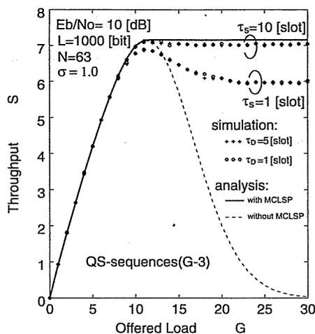
Fig. 8 Throughput performance of CDMA slotted ALOHA systems with MCLSP.
