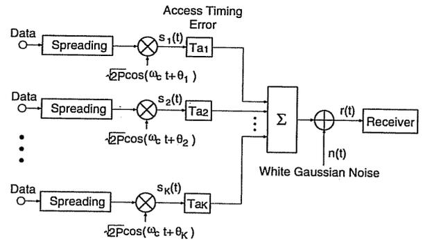
Fig. 3 Model of transmitter and receiver.
