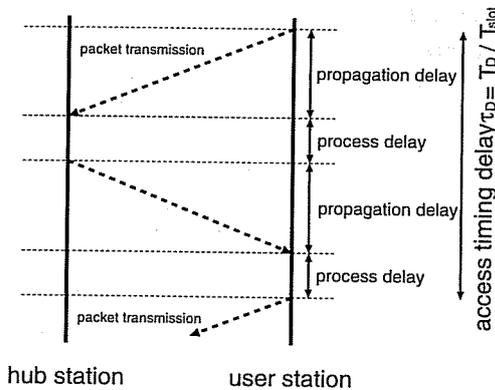
Fig. 2 Access timing delay.
