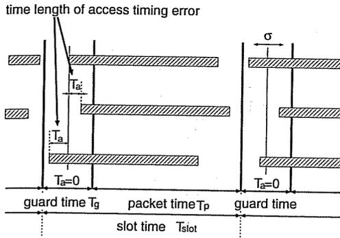
Fig. 1 Model of channel status of CDMA slotted ALOHA system.
