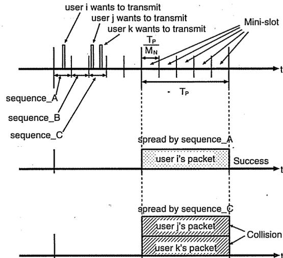
Fig. 5 Sequence allocation and collision of sequence (guard time is omitted).
