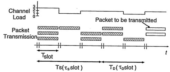
Fig. 6 Model of CDMA slotted ALOHA systems with MCLSP.
