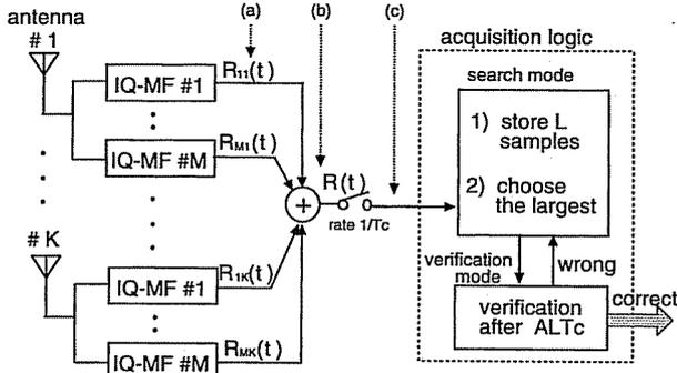
Fig. 3 Acquisition circuit.
