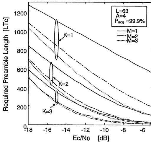
Fig. 8 Required preamble length.
