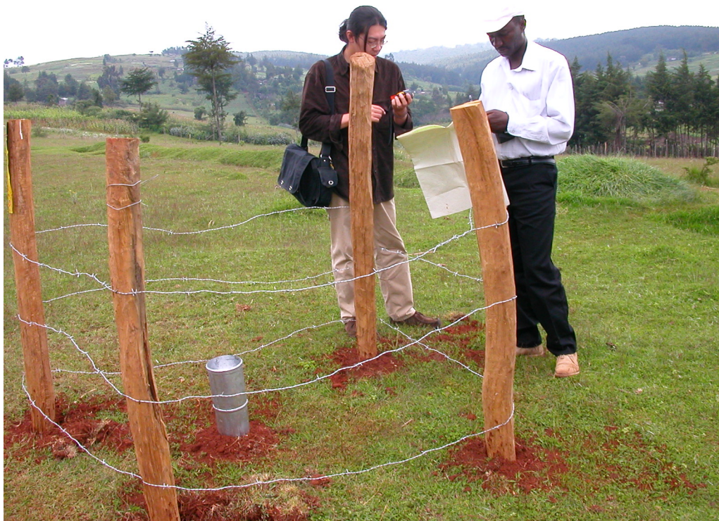
Plate IV-1. A newly installed rain gauge in the schoolyard, Kericho. (August 2003)
