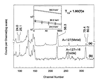
FIG. 4. Comparison of the  $\gamma$ -ray spectra obtained with a metallic beam [A = 127 (a)] and an oxide beam [A = 127 + 16 (b)]. The inset shows decay curves of the 80.2-, 56.3-, and 24.0-keV  $\gamma$  rays of the <sup>127m</sup>Ba isomeric transitions.
