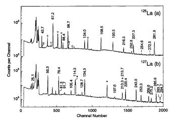
FIG. 1. Low energy portions of the  $\gamma$ -ray spectra in the decay of <sup>125</sup>La (a) and <sup>127</sup>La (b) obtained with a LEPS. The open and closed circles indicate the  $\gamma$  rays associated with the decay of their daughter or granddaughter nuclei, respectively.
