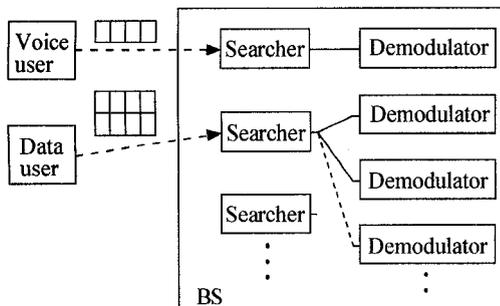
Fig. 2. Common searcher configuration for integrated traffic.
