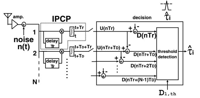
Fig. 5. The block diagram of differential IPCP.
