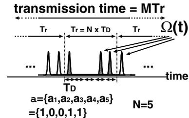
Fig. 1. The transmission signal ( $N=5$ ).
