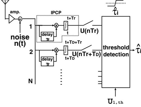
Fig. 4. The block diagram of parallel IPCP receiver.
