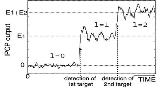
Fig. 3. The output of the IPCP receiver.
