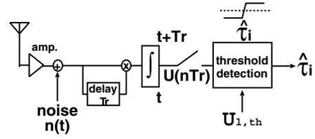
Fig. 2. The block diagram of IPCP receiver.
