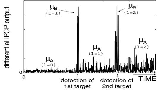
Fig. 6. The parallel differential IPCP receiver output.
