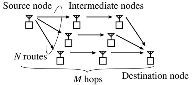
Fig. 1. Wireless multi-hop network model.
