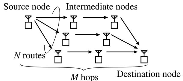
Fig. 1. Wireless multi-hop network model.
