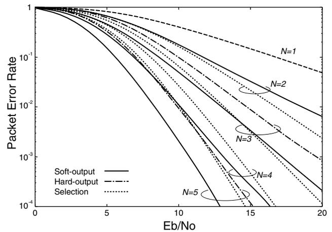
Fig. 8. Packet error rate versus  $E_b/N_0$  ( $M = 2$ , slow Rayleigh fading).
