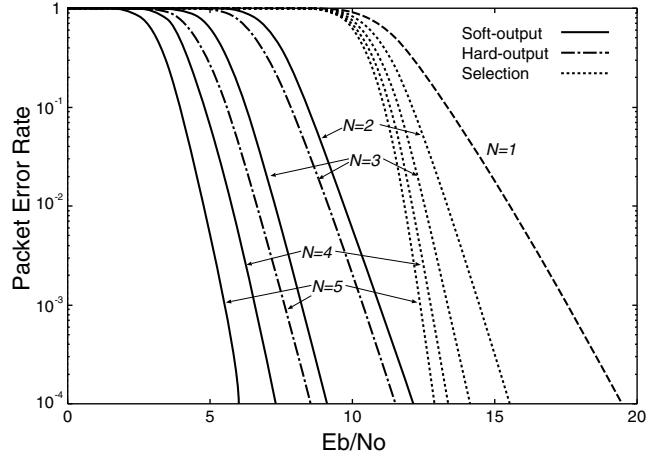
Fig. 4. Packet error rate versus  $E_b/N_0$  ( $M = 2$ , fast Rayleigh fading).
