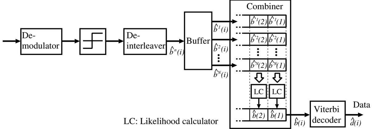
Fig. 3. Receiver structure.
