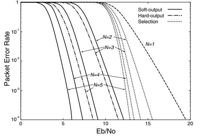
Fig. 4. Packet error rate versus  $E_b/N_0$  ( $M = 2$ , fast Rayleigh fading).
