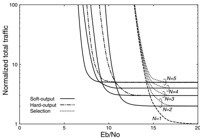
Fig. 7. Total traffic versus  $E_b/N_0$  ( $M = 4$ , fast Rayleigh fading).
