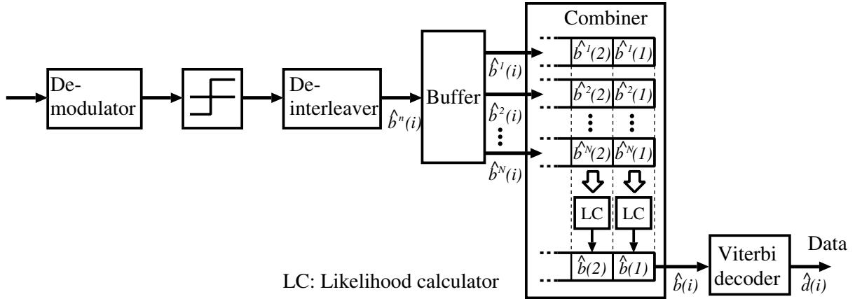
Fig. 3. Receiver structure.
