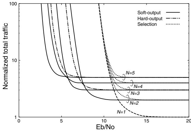
Fig. 6. Total traffic versus  $E_b/N_0$  ( $M = 2$ , fast Rayleigh fading).
