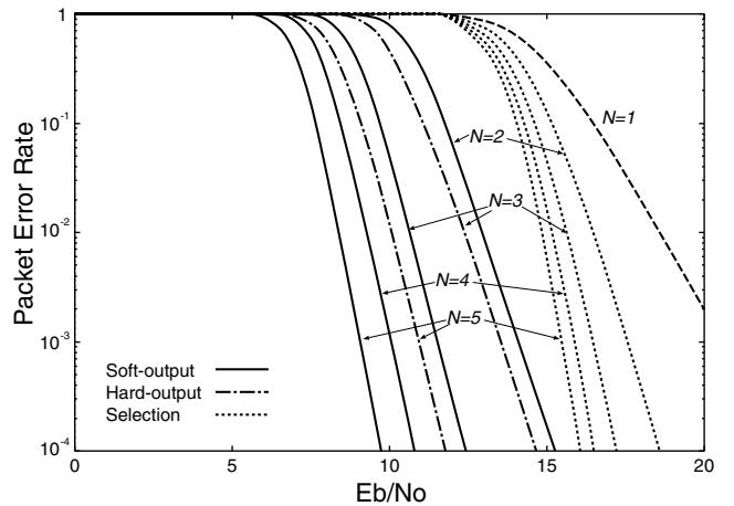
Fig. 5. Packet error rate versus  $E_b/N_0$  ( $M = 4$ , fast Rayleigh fading).
