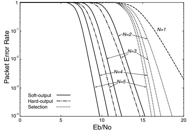
Fig. 5. Packet error rate versus  $E_b/N_0$  ( $M = 4$ , fast Rayleigh fading).
