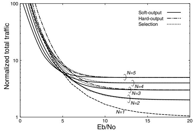
Fig. 9. Total traffic versus  $E_b/N_0$  ( $M = 2$ , slow Rayleigh fading).
