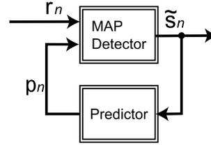
Figure 1: Concept of the new MAP receiver
