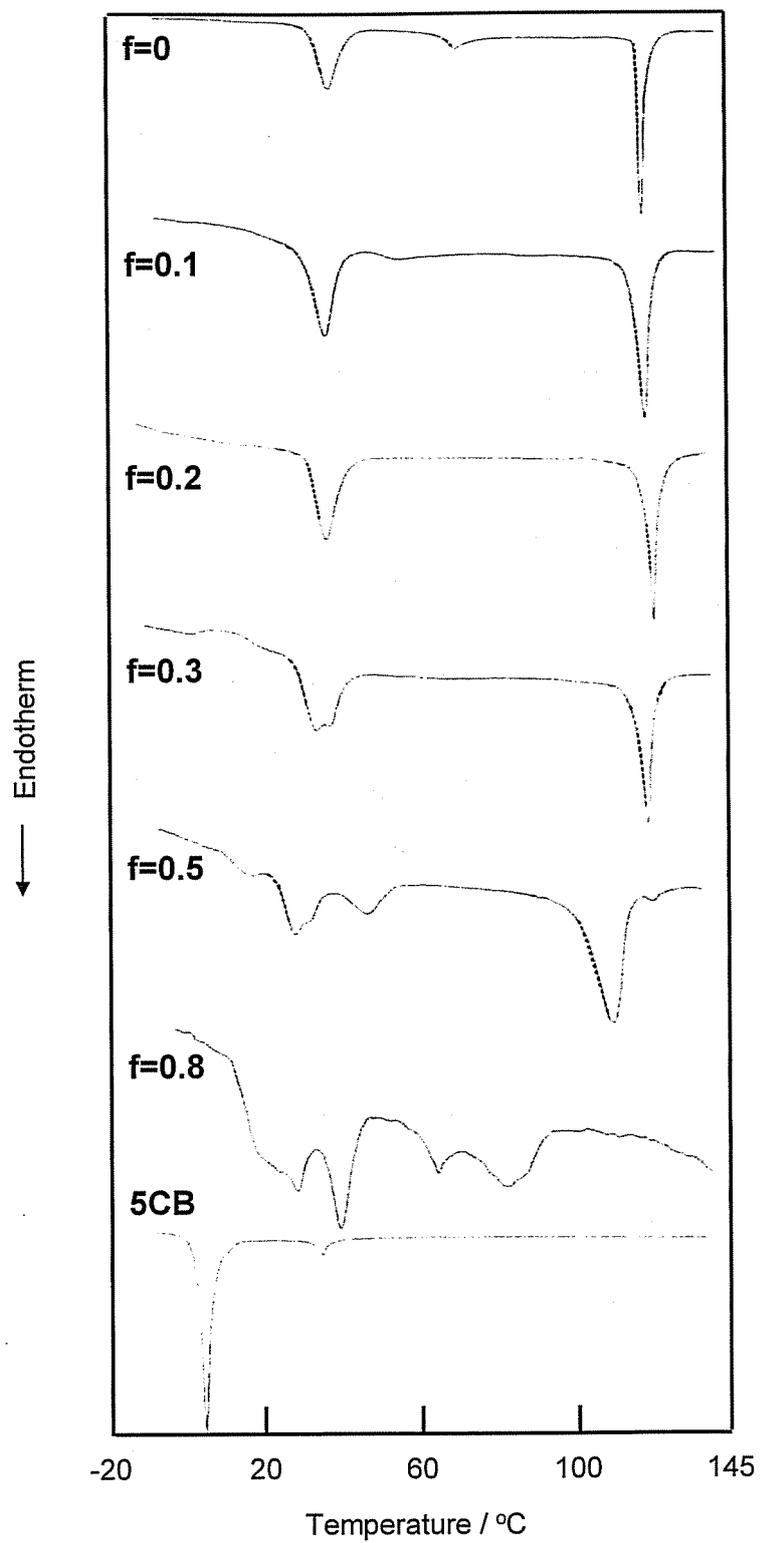
**Figure 3-2** DSC curves of p(EO114-Az67)/5CB hybrids at various molar fractions of p(EO114-Az67) and 5CB ( $f$ ).
