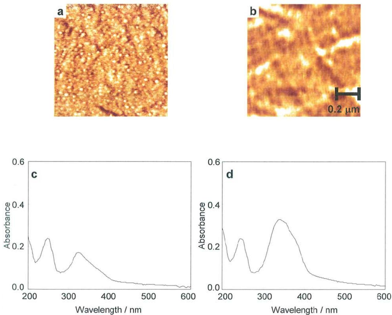
**Figure 2-13.** The orientation of PEO cylinders and Az mesogens in the  $p(\text{EO}_{114}\text{-Az}_{67})$  films on chemically patterned substrate surfaces. **a** and **b**, Phase-mode AFM images ( $1\ \mu\text{m} \times 1\ \mu\text{m}$ ) at the areas of different chemical nature (**a**: non UV irradiated and **b**: UV irradiated) after post-treatment. **c** and **d**, UV-visible absorption spectra at the each area of the corresponding film.
