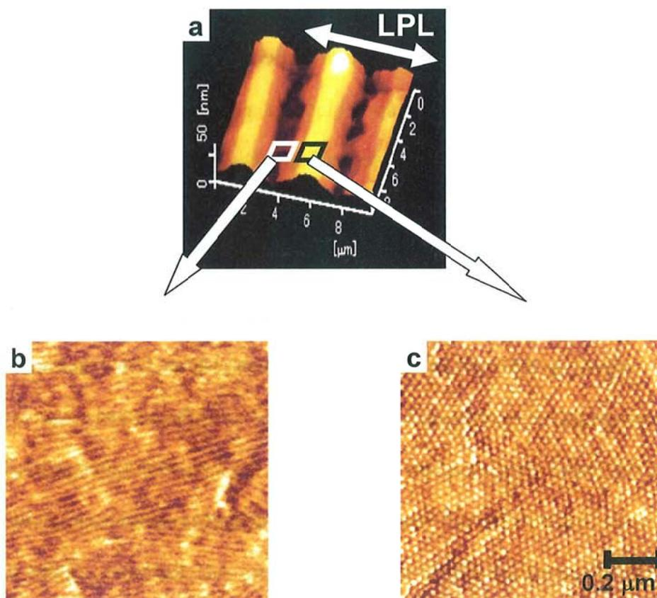
**Figure 4-1.** AFM images of surface relief structure of p(EO<sub>114</sub>-Az<sub>67</sub>) film after post-treatment. Topographic AFM image (10 x 10 μm) of a photogenerated relief (a), and corresponding magnified phase mode images (0.8 x 0.8 μm) at the trough (b) and crest (c) resulted from (*s*-: *s*-) mode holographic irradiation at 400 mJ cm<sup>-2</sup>.
