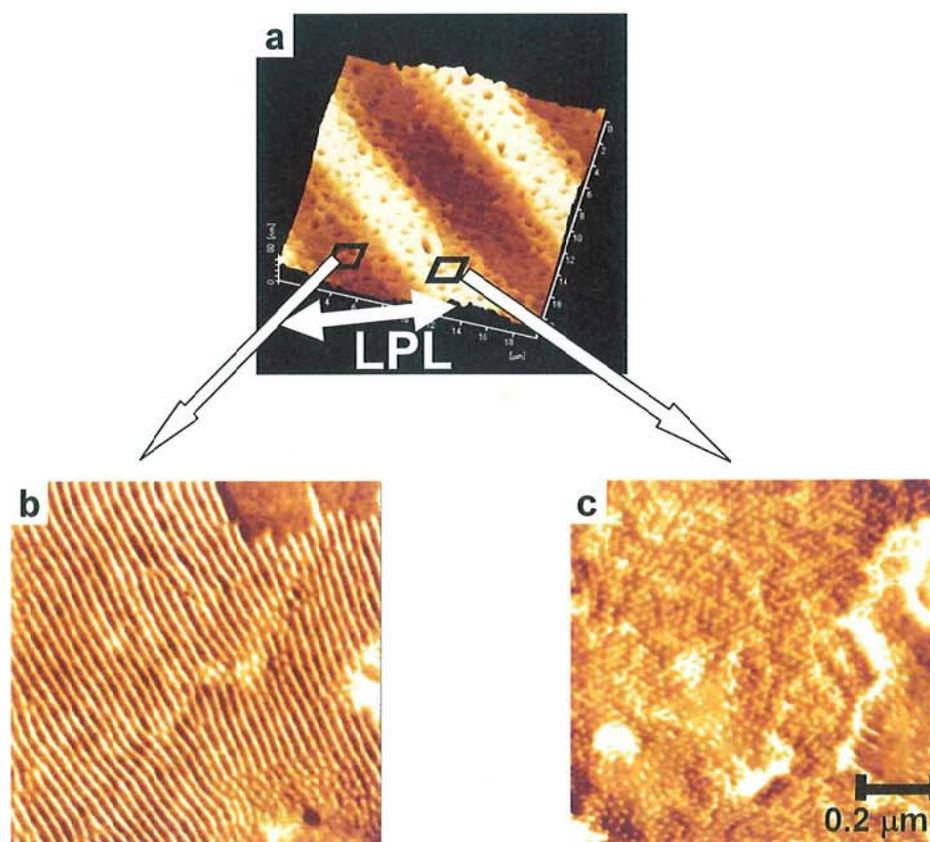
**Figure 4-7.** AFM images of the surface relief structure of the p(EO<sub>114</sub>-Az<sub>67</sub>) film after post-treatment. Topographic AFM image (10 x 10 μm) of a photogenerated relief (a), and corresponding magnified phase mode images (1.0 x 1.0 μm) at the trough (b) and crest (c) resulted from irradiation through a line and space photomask at 5 J cm<sup>-2</sup>.
