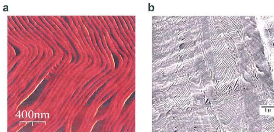
**Figure 1-7** (a) AFM phase image of stripe morphological feature of a block copolymer film. (b) SEM micrograph showing selective deposition of Pd nanoparticles onto the stripe morphological feature after the metallization process. (taken from Ref. 24)
