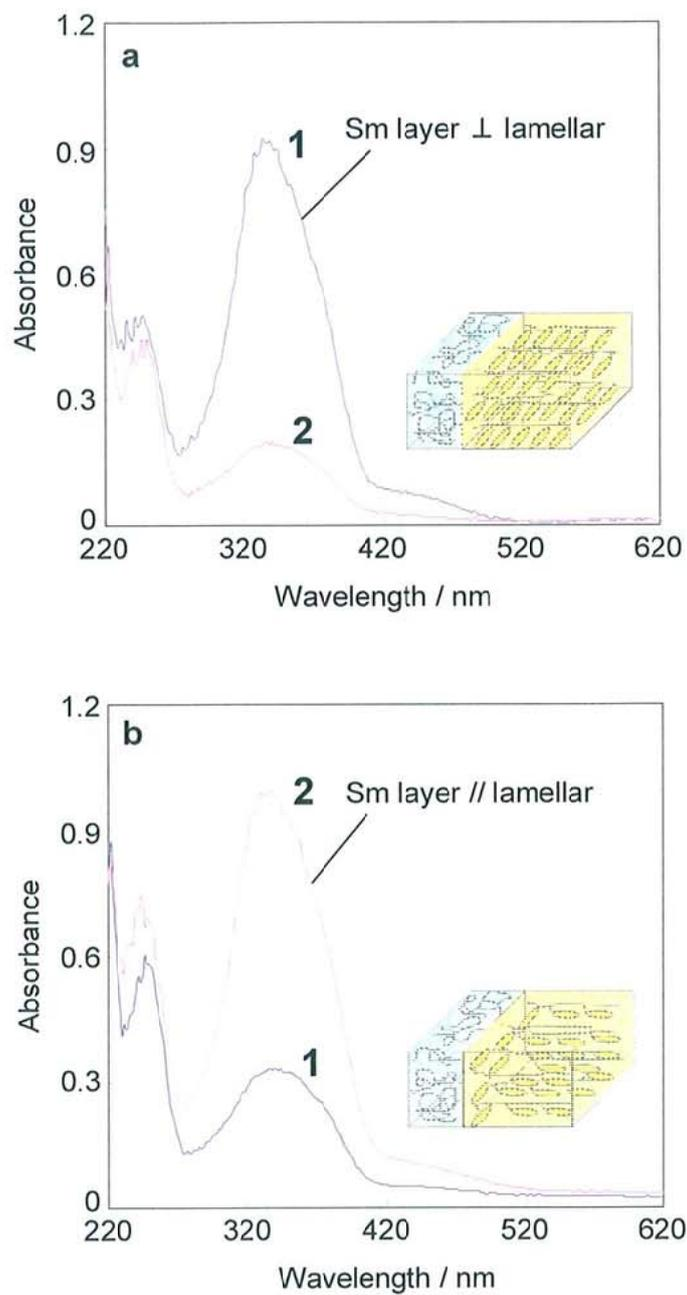
**Figure 6-6** UV-vis absorption spectra of the initial (a) and subsequently LPL-irradiated (b) films. **1** and **2** display polarized spectra taken with probing beam parallel and perpendicular to the direction of the lamellar structure. Schematic illustrations of the corresponding hierarchical structures are inserted in **a** and **b**.
