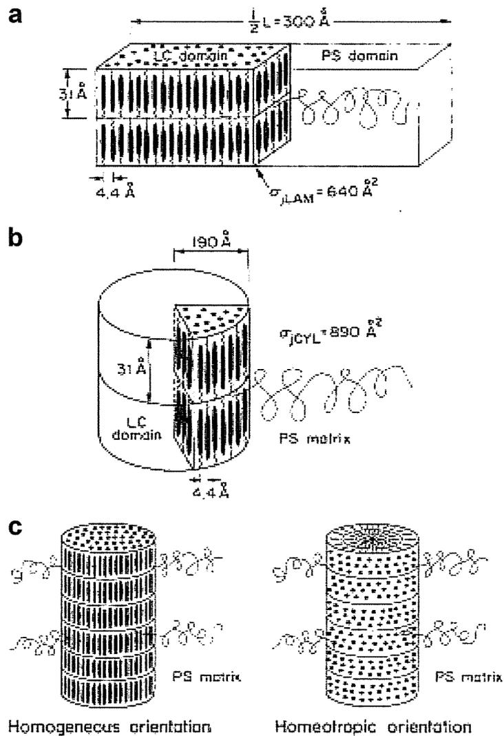
**Figure 1-2** (a) Schematic illustration of lamellar structure of LC-segment-containing block copolymers. (b and c) cylinder structures (homogeneous and homeotropic orientation of mesogens to the IMDS). (taken from Ref. 4)
