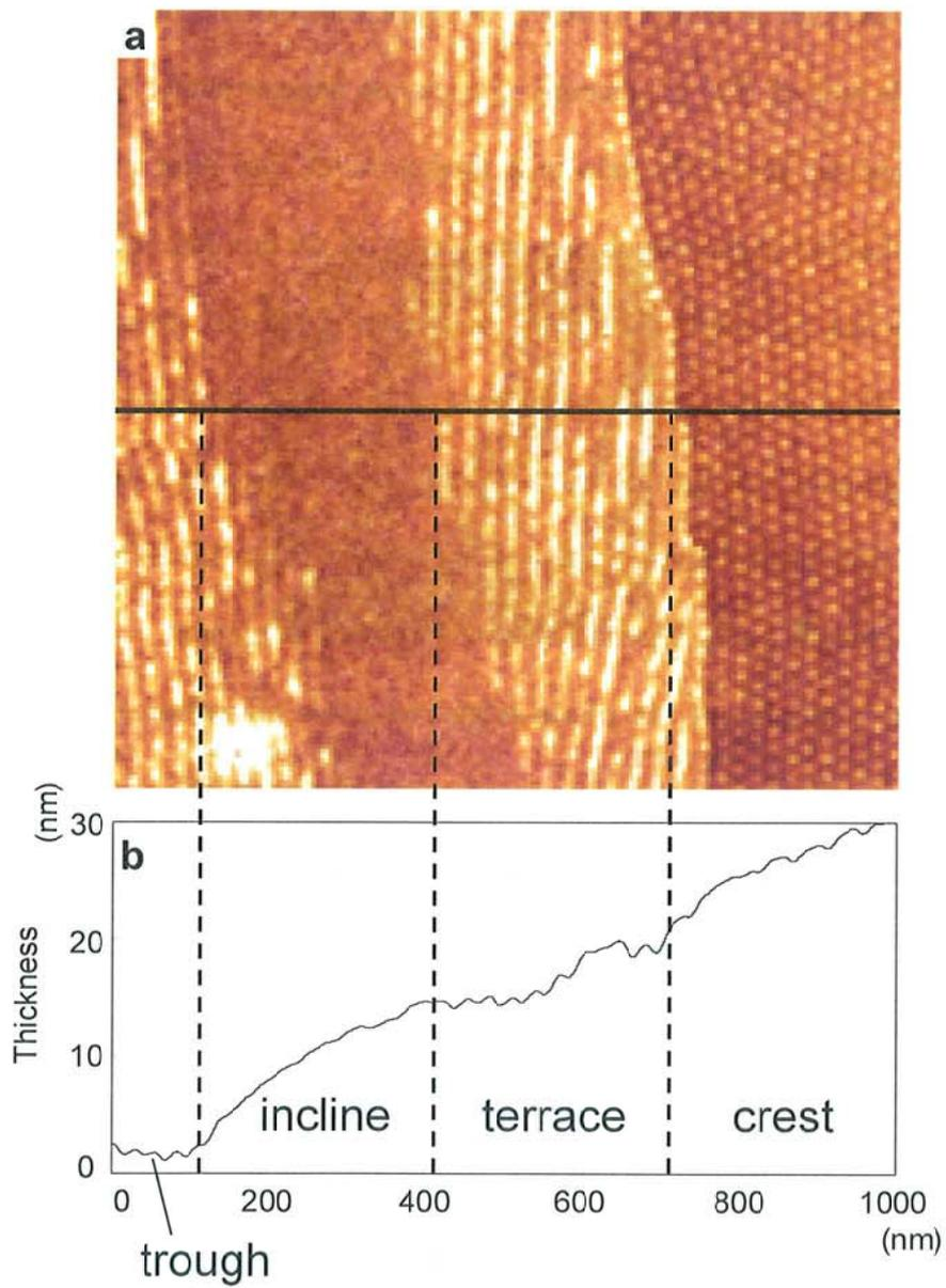
**Figure 4-4.** AFM data of the surface relief structure at the boundary region of the  $p(\text{EO}_{114}\text{-Az}_{67})$  film after post-treatment. Phase mode AFM image ( $1 \times 1 \mu\text{m}$ ) of the photogenerated relief (a), and cross section of the topographic AFM image corresponding to the black line indicated in a (b).
