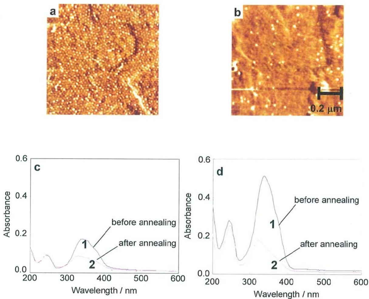
**Figure 2-10.** The orientation of PEO cylinders and Az mesogens in the p(EO<sub>114</sub>-Az<sub>67</sub>) films on OTS-modified substrate surfaces. a and b, Phase-mode AFM images (1 μm x 1 μm) with different film thickness (a: 50 nm and b: 90 nm) after post-treatment. c and d, UV-visible absorption spectra of the corresponding films for as-cast (1) and after annealing (2).
