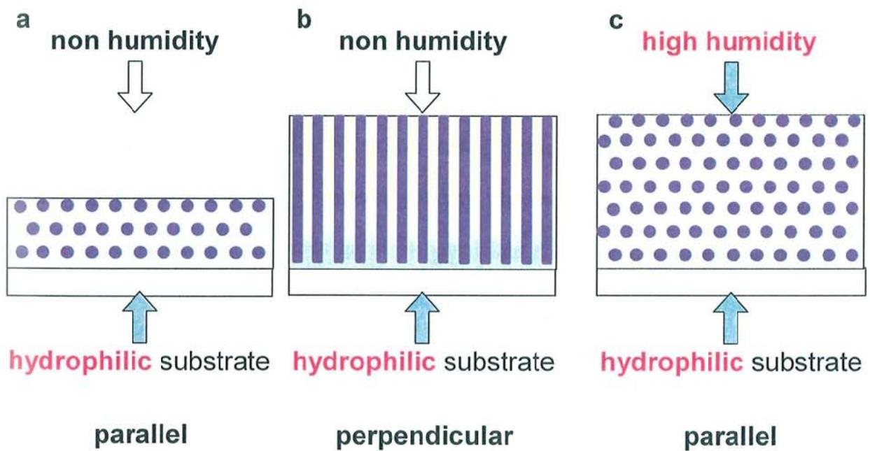
**Figure 2-6.** Schematic illustration of the relation between the direction of cylinder orientation and the annealing condition in the p(EO<sub>114</sub>-Az<sub>67</sub>) films with different thickness. (a) the cylinder orientation in thinner film after annealing under normal atmosphere. **b** and **c** the cylinder orientation in thicker film after annealing under normal or humidified atmosphere.
