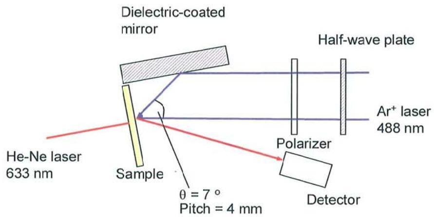
**Figure 3-1** Schematic illustration of the experimental setup for the holographic recording by an argon ion laser beam.
