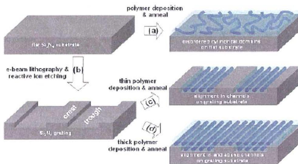
**Figure 1-4** Schematic illustration of alignment control process of cylindrical nanodomains by utilizing topographical patterned substrate. (taken from Ref. 14)
