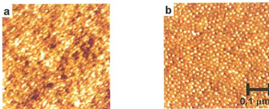
**Figure 2-3.** Phase-mode AFM images ( $0.5\ \mu\text{m} \times 0.5\ \mu\text{m}$ ) of the  $\text{p}(\text{EO}_{40}\text{-Az}_{44})$  films with different film thickness: 60 nm (a) and 70 nm (b) after annealing.
