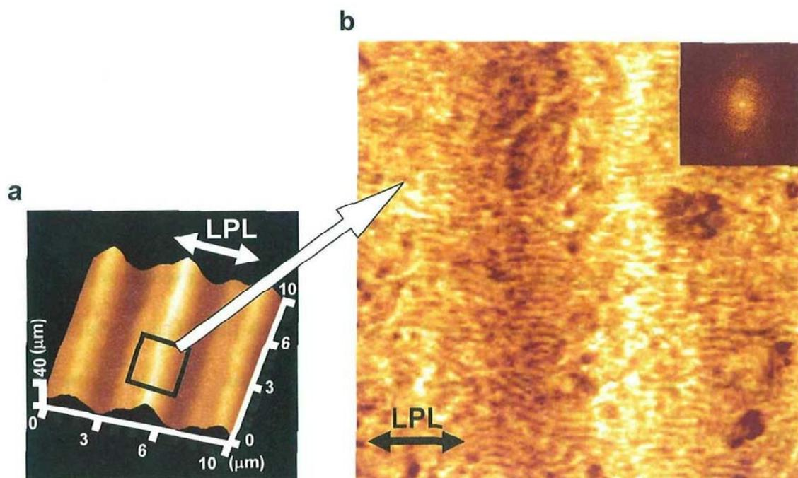
**Figure 6-8** AFM image of the  $p(S_{226}\text{-Az}_{56})$  film after interferometric irradiation with ( $p$ -:  $p$ -) mode  $\text{Ar}^+$  laser beam. Topographic AFM image (a,  $10 \times 10 \mu\text{m}$ ) of a photogenerated relief and a magnified phase mode image (b,  $3.0 \times 3.0 \mu\text{m}$ ) of hill to valley slope area. Fast Fourier transform spectrum is shown in b.
