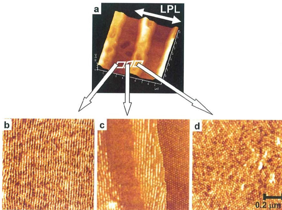
**Figure 4-3.** AFM images of the surface relief structure of the p(EO<sub>114</sub>-Az<sub>67</sub>) film after post-treatment. Topographic AFM image (10 x 10 μm) of a photogenerated relief (a), and corresponding magnified phase mode images (1.0 x 1.0 μm) at the trough (b), boundary region (c) and crest (d) resulted from the (*p*-: *p*-) mode holographic irradiation at 5 J cm<sup>-2</sup>.
