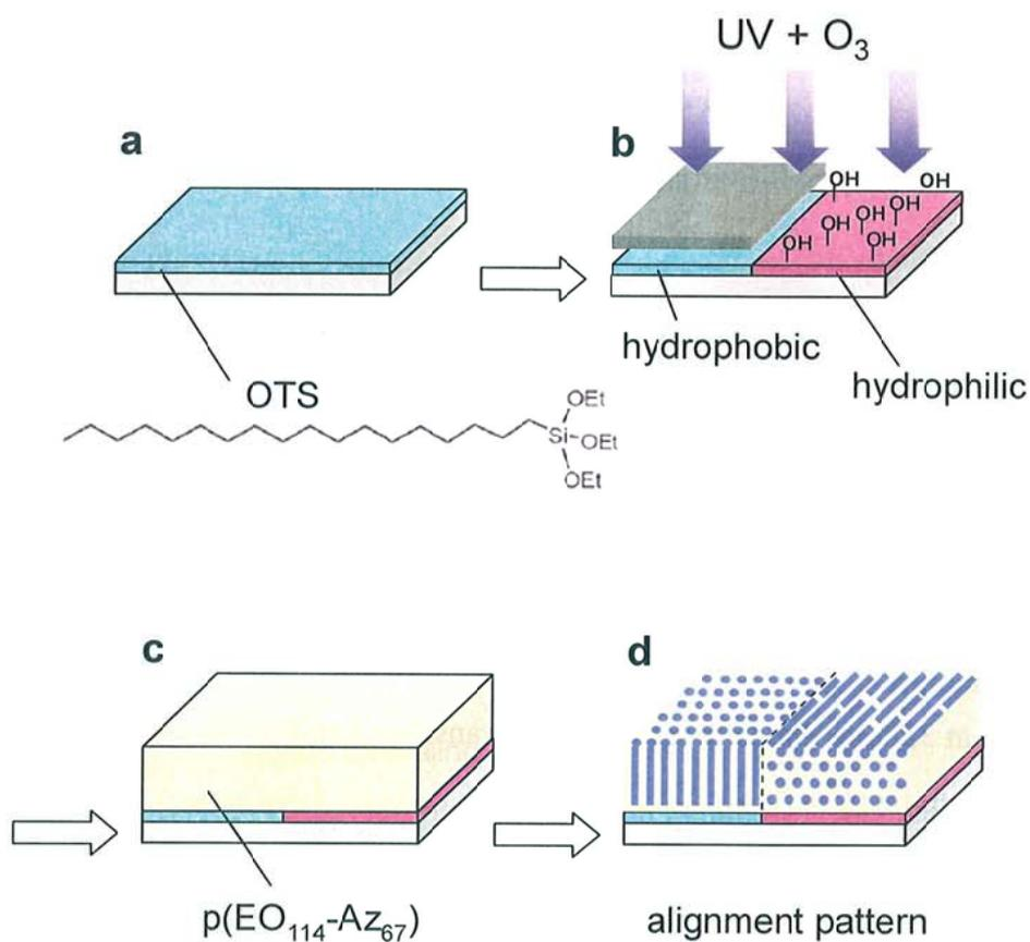
**Figure 2-12.** Schematic illustration of the strategy for patterning of chemically nature of OTS-modified substrate surface. (a) An OTS film on cleaned quartz glass substrate. (b) Exposure to UV light and  $O_3$  atmosphere through a mask. (c) Spincoating of the  $p(EO_{114}-Az_{67})$  film on a resulting substrate. (d) Alignment pattern of cylinders after post-treatment.
