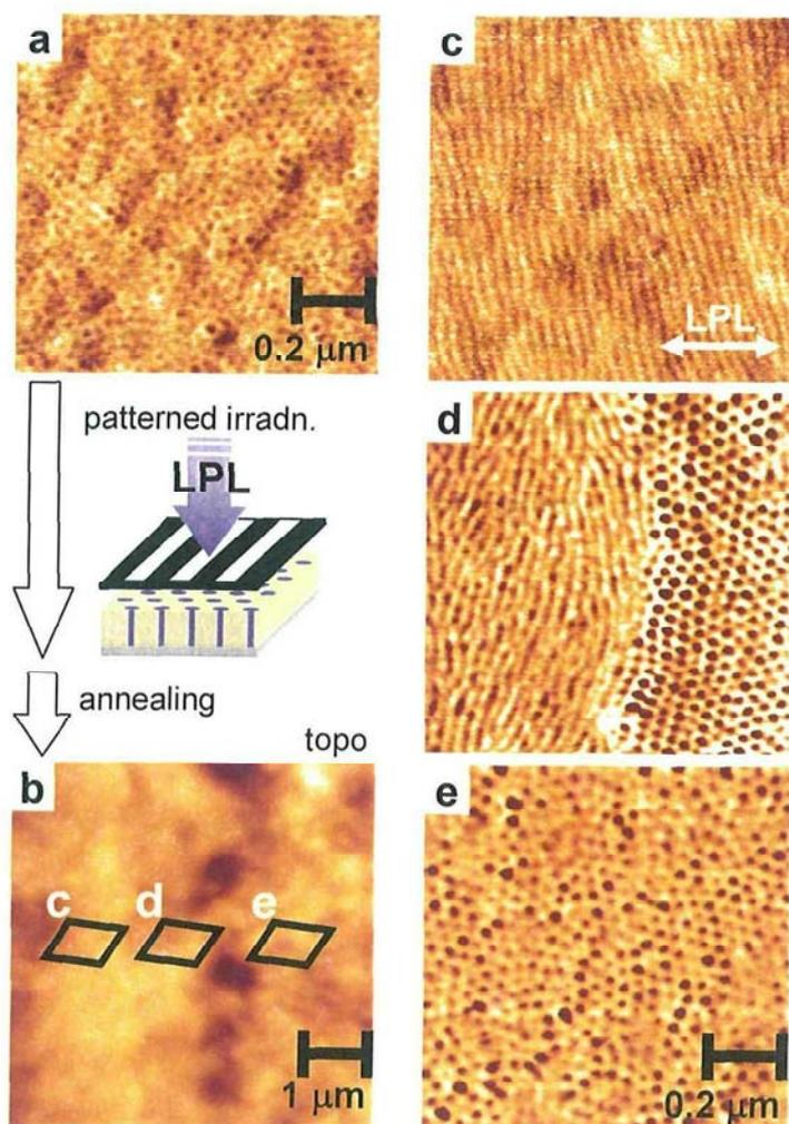
**Figure 5-6** Orientational control of PS cylinder by patterned irradiation of LPL (436 nm) in p(S76-Az140) film (thickness = ca. 100 nm). (a) The initial state where all cylinders were in the perpendicular orientation. (b) Topographical AFM image after patterned irradiation with LPL. (c – e) Phase mode AFM images taken at the irradiated area (c), boundary region (d), and non-irradiated area (e).
