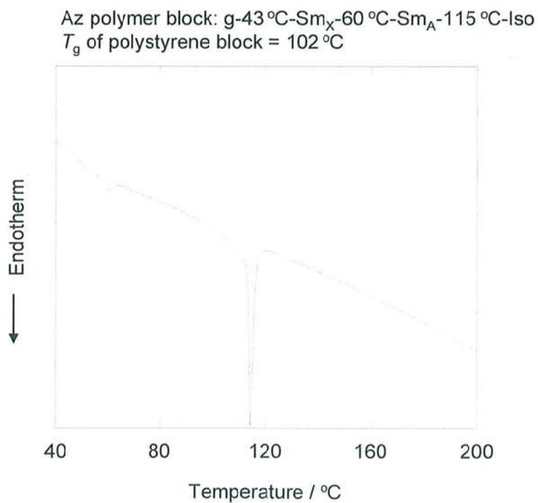
Figure 6-2 DSC chart of the p(S<sub>226</sub>-Az<sub>56</sub>) in a heating process. Heating rate: 10 °C/min.
