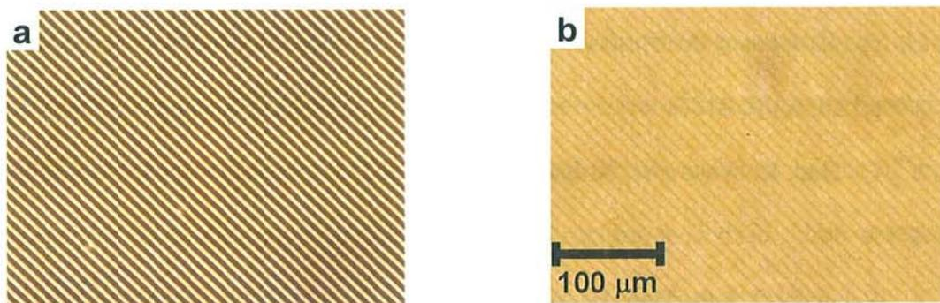
**Figure 3-9** Microphotograph of a photomask (a) and the relief structure resulted from exposure to visible light through a photomask (b) in the p(EO114-Az67)/5CB hybrid film ( $f = 0.5$ ).
