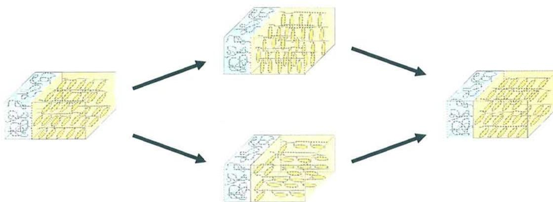
**Figure 6-5** Schematic illustration of the orientation of mesogenic Az group confined in lamellar structure of  $p(S_{226}\text{-Az}_{56})$  film in the series of irradiation processes indicated in Figure 6-3. The upper and lower routes show the out-of-plane and in-plane photoinduced reorientation of the LC block, respectively.
