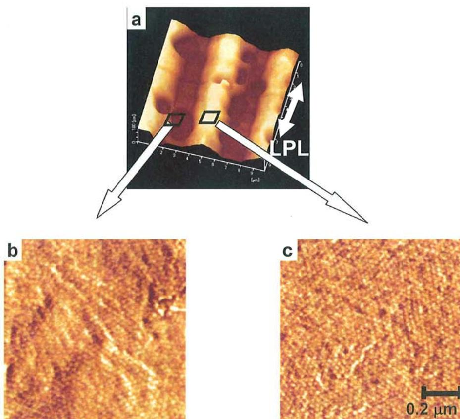
**Figure 4-5.** AFM images of the surface relief structure of the p(EO<sub>114</sub>-Az<sub>67</sub>) thick film after post-treatment. Topographic AFM image (10 x 10 μm) of the photogenerated relief (a), and corresponding magnified phase mode images (0.8 x 0.8 μm) at the trough (b) and crest (c) resulted from the (s-: s-) mode holographic irradiation at 400 mJ cm<sup>-2</sup>.
