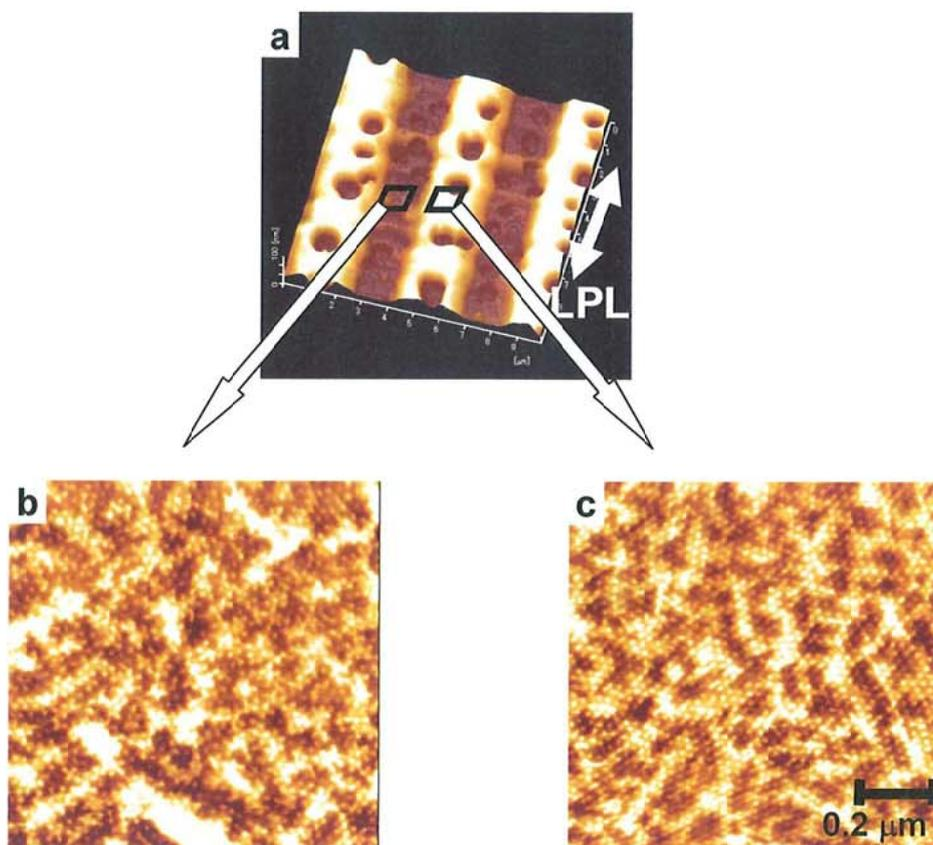
**Figure 4-6.** AFM images of the surface relief structure of the p(EO<sub>114</sub>-Az<sub>67</sub>) film on a hydrophobic substrate after post-treatment. Topographic AFM image (10 x 10 μm) of the photogenerated relief (a), and corresponding magnified phase mode images (1.0 x 1.0 μm) at the trough (b) and crest (c) resulted from the (s-: s-) mode holographic irradiation at 400 mJ cm<sup>-2</sup>.
