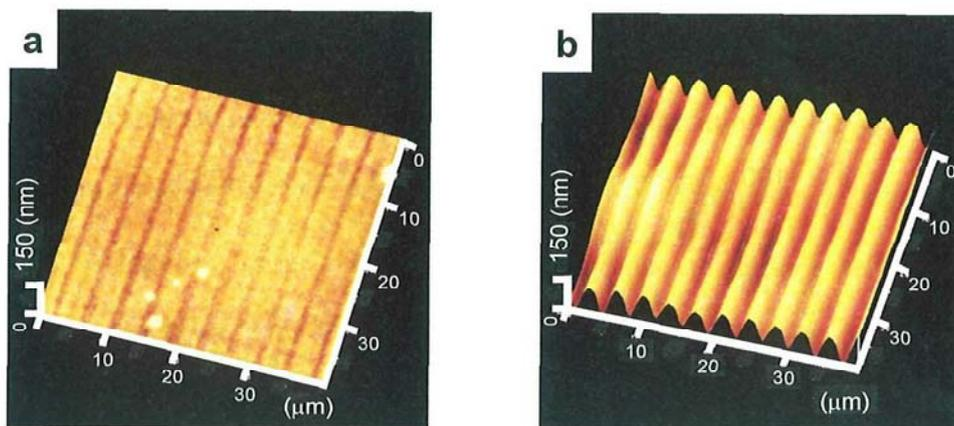
**Figure 3-5** Topographic AFM images (40 x 40 mm) of photogenerated relief structure in (a) the pure p(EO114-Az67) film and (b) the p(EO114-Az67)/5CB hybrid film ( $f = 0.5$ ).
