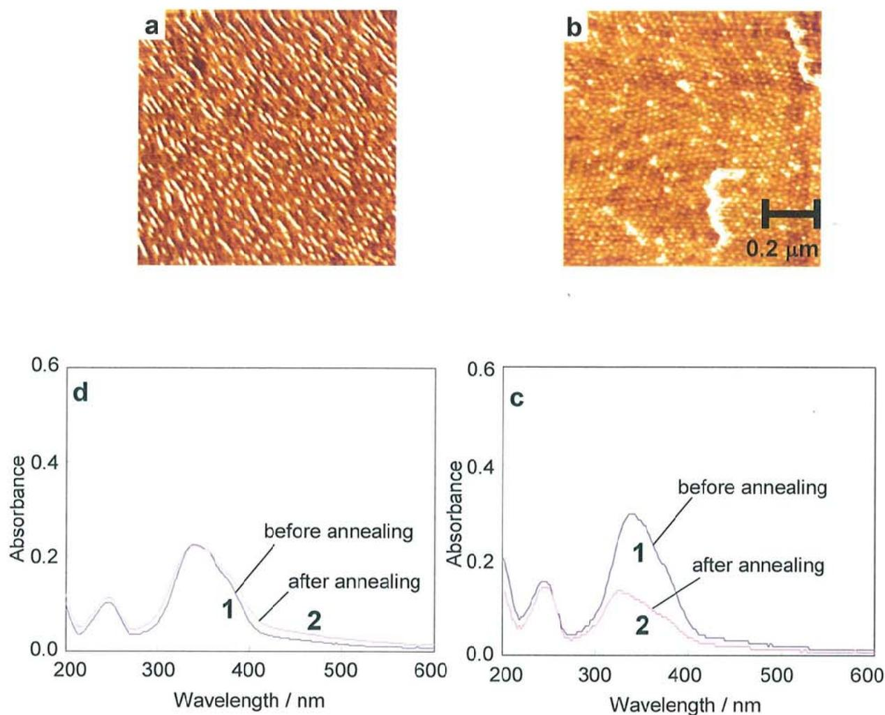
**Figure 2-11.** The orientation of PEO cylinders and Az mesogens in the p(EO<sub>114</sub>-Az<sub>67</sub>) films on OTS-modified substrate surfaces exposed to UV light and O<sub>3</sub> atmosphere . a and b, Phase-mode AFM images (1 μm x 1 μm) with different film thickness (a: 50 nm and b: 70 nm) after post-treatment. c and d, UV-visible absorption spectra of the corresponding films for as-cast (1) and after annealing (2).
