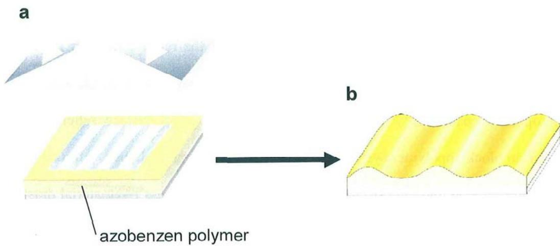
**Figure 1-9** Schematic illustration of photo-triggered mass migration. (a) Interference exposure with LPL. (b) resulting surface relief structure.
