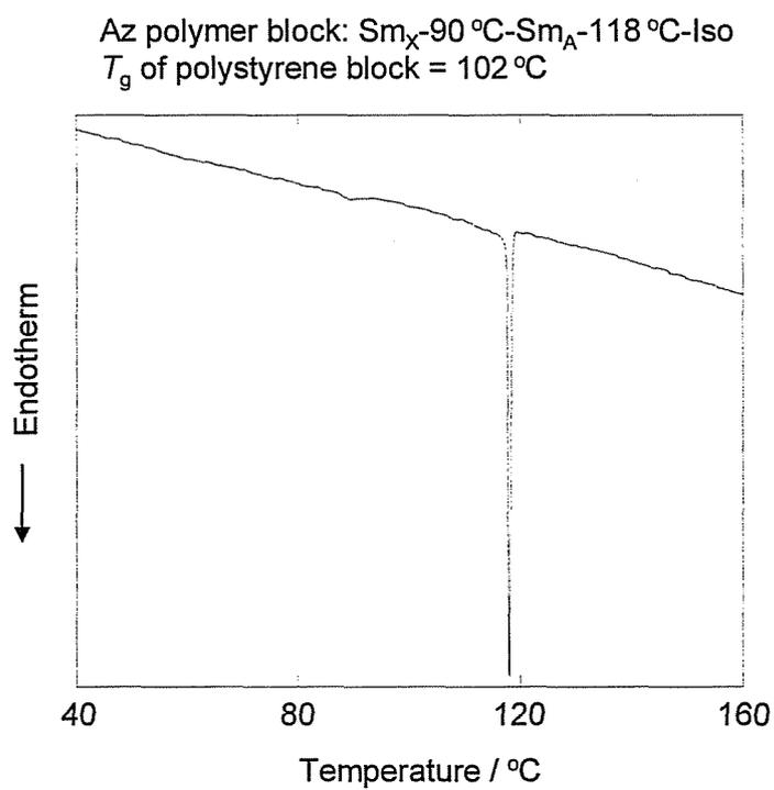
**Figure 5-4** DSC chart of the p(S<sub>76</sub>-Az<sub>140</sub>) in a heating process. Heating rate: 10 °C/min.
