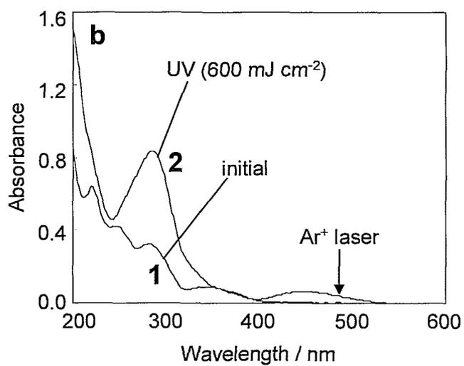
**Figure 3-3** UV-visible absorption spectra. p(EO114-Az67) film (a) and the p(EO114-Az67)/5CB hybrid film ( $f = 0.5$ ) (b) before (1) and after UV light exposure (2).
