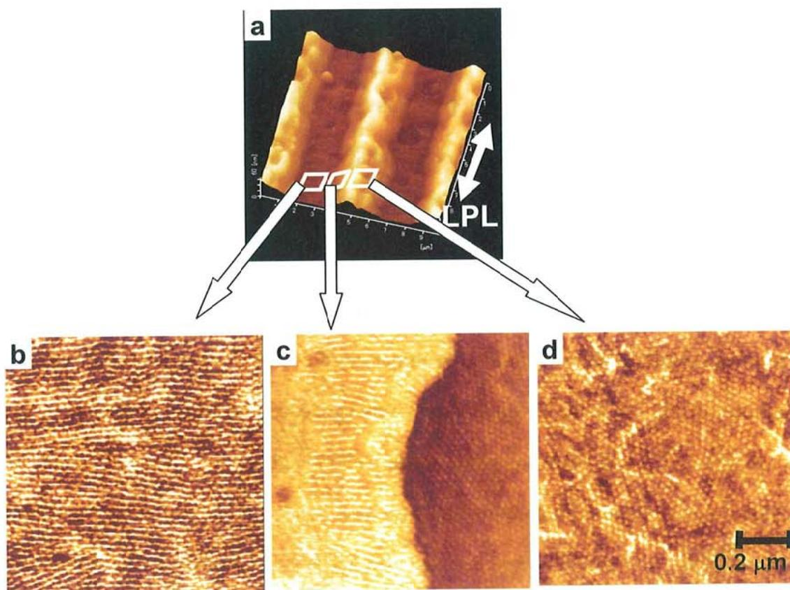
**Figure 4-2.** AFM images of the surface relief structure of the p(EO<sub>114</sub>-Az<sub>67</sub>) film after post-treatment. Topographic AFM image (10 x 10 μm) of a photogenerated relief (a), and corresponding magnified phase mode images (1.0 x 1.0 μm) at the trough (b), boundary region (c) and crest (d) resulted from the (s-: s-) mode holographic irradiation at 5 J cm<sup>-2</sup>.
