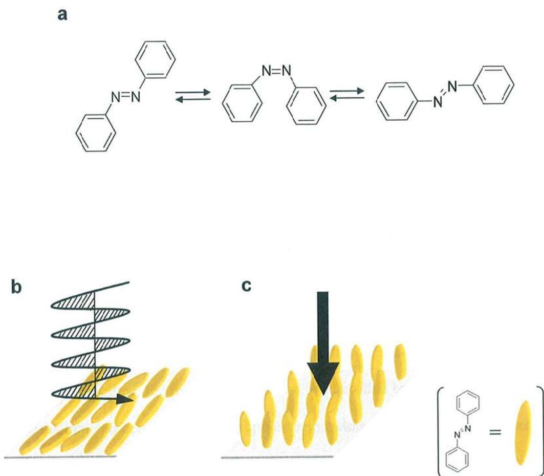
**Figure 1-8** (a) Schematic illustration of photoisomerization of azobenzene. (b) In-plane alignment of Az by LPL irradiation. (c) Out-of-plane alignment of Az by non-LPL irradiation from the normal direction to the film surface.
