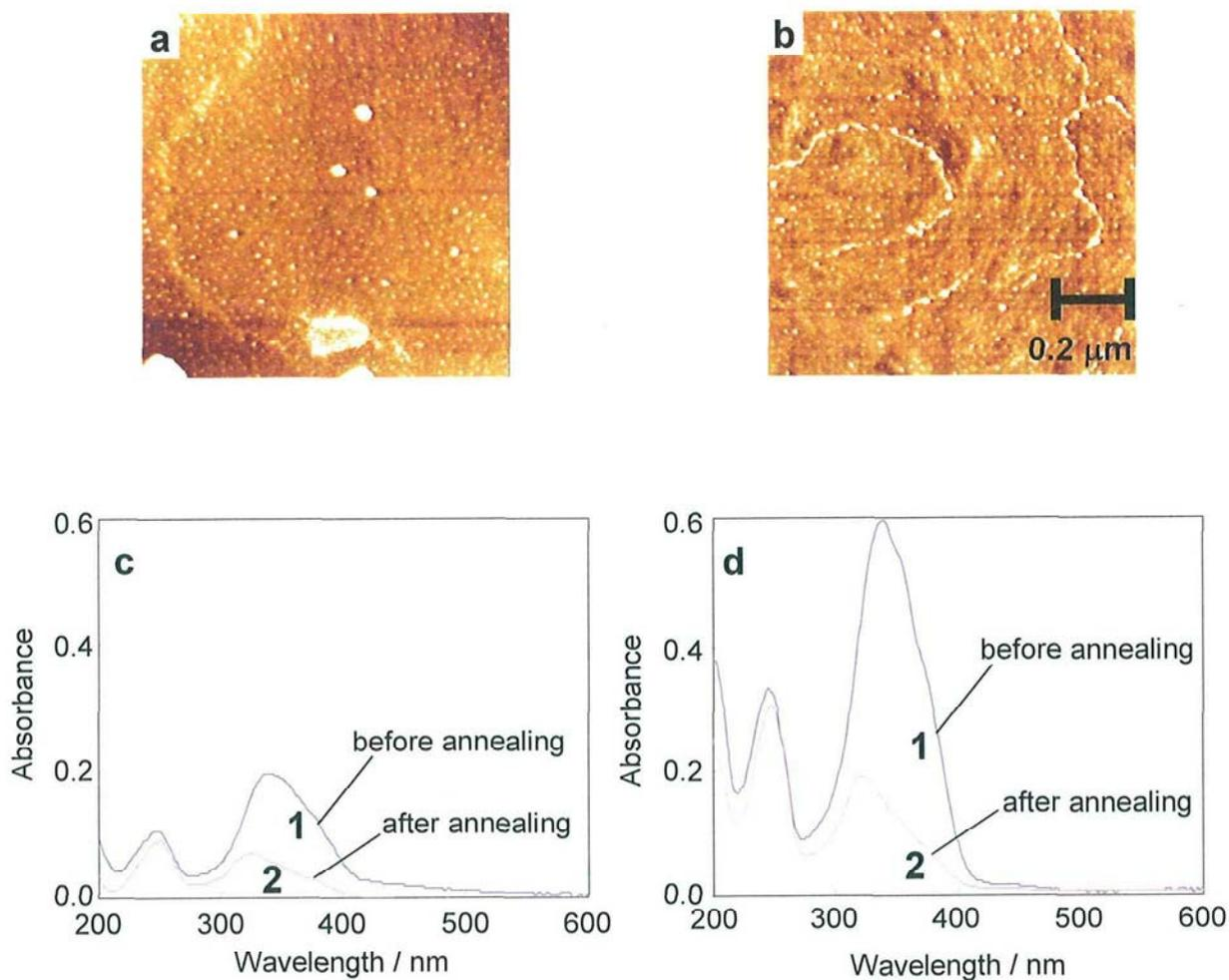
**Figure 2-9.** The orientation of PEO cylinders and Az mesogens in the p(EO<sub>114</sub>-Az<sub>67</sub>) films on HMDS-modified substrate surfaces. **a** and **b**, Phase-mode AFM images (1 μm x 1 μm) with different film thickness (**a**: 30 nm and **b**: 90 nm) after post-treatment. **c** and **d**, UV-visible absorption spectra of the corresponding films for as-cast (1) and after annealing (2).
