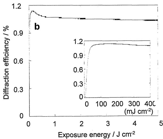
**Figure 3-7** First-order diffraction efficiency of the  $p(\text{EO}_{114}\text{-Az}_{87})/5\text{CB}$  hybrid films resulted from (a) ( $p$ -:  $p$ -) mode or (b) ( $s$ -:  $s$ -) mode holographic irradiation.
