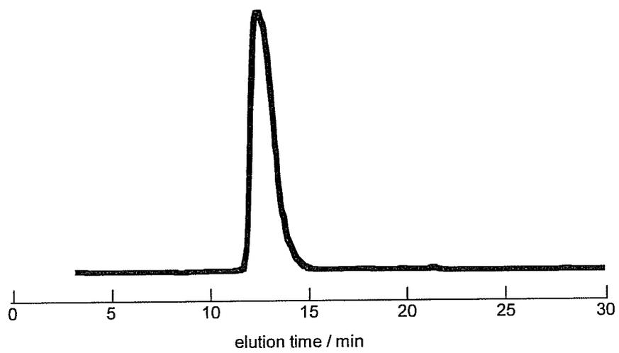
Figure 5-2 GPC chart of p(S<sub>76</sub>-Az<sub>140</sub>).
