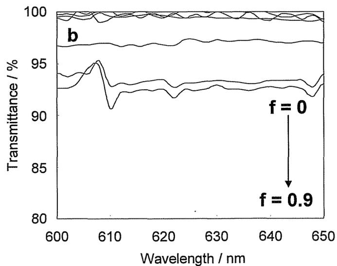
**Figure 3-6** (a) The first-order diffraction efficiency (○) and surface modulation depth (■) of the p(EO114-Az67)/5CB hybrid films with various 5CB fractions ( $f$ ). (b) Visible transmission spectra of the p(EO114-Az67)/5CB hybrid films with various 5CB fractions ( $f$ ).
