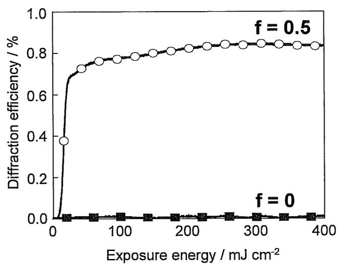
**Figure 3-4** First-order diffraction efficiency of the p(EO114-Az67) film (■) and the p(EO114-Az67)/5CB hybrid film ( $f = 0.5$ ) (○) vs exposure energy.
