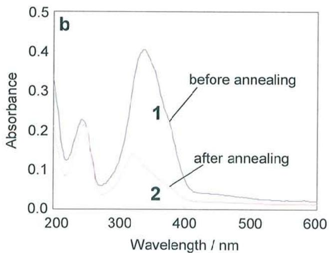
**Figure 2-5.** UV-visible absorption spectra of the corresponding p(EO<sub>40</sub>-Az<sub>44</sub>) films are shown: 60 nm (a) and 70nm thickness (b) for as-cast (1) and after annealing (2).
