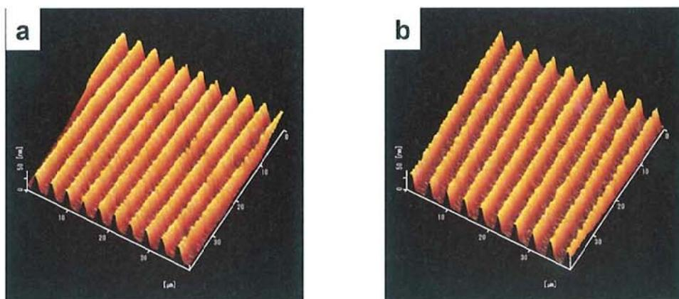
**Figure 3-8** Topographic AFM images (40 x 40 μm) of photogenerated relief structure resulted from (a) (p-: p-) mode or (b) (s-: s-) mode holographic irradiation in the p(EO114-Az67)/5CB hybrid film ( $f = 0.5$ ).
