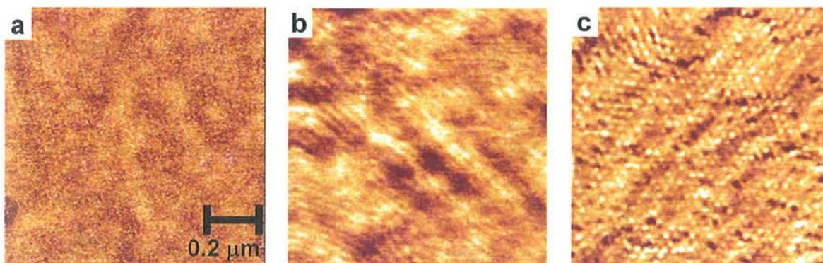
**Figure 2-2.** Phase-mode AFM images ( $1\ \mu\text{m} \times 1\ \mu\text{m}$ ) of the  $\text{p}(\text{EO}_{114}\text{-Az}_{67})$  films with different film thickness: 20 nm (a), 60 nm (b) and 70 nm (c) after annealing.
