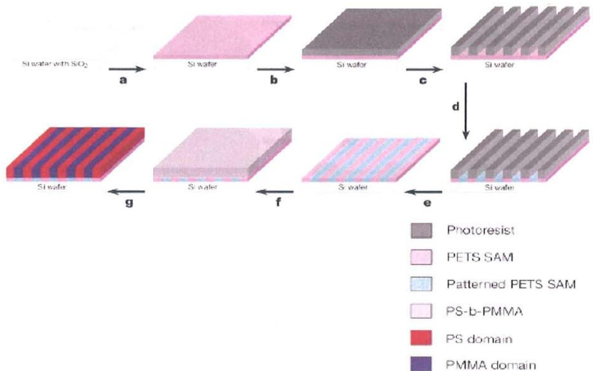
**Figure 1-5** Schematic illustration of the strategy used to create chemically patterned surfaces and investigate the epitaxial assembly of nanodomains. (taken from Ref. 18)
