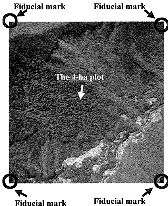
Fig. 1. A natural color aerial photograph of the Tatera Forest Reserve. This aerial photograph was transformed into a digital orthophoto. The 4-ha plot was included in a white frame. The plot is in the center of the white frame. Fiducial marks are in the four corners. The intersection of the diagonal lines between the fiducial marks is the projection center.
