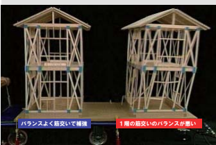
木造家屋の倒壊実験用モデル Models of Wooden Houses for Realistic Response & Collapse
