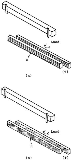
Fig. 1. Specimen & Loading condition I.
