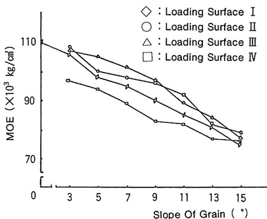
Fig. 12. Modulus of Elasticity for Four Different Loading Surfaces.
