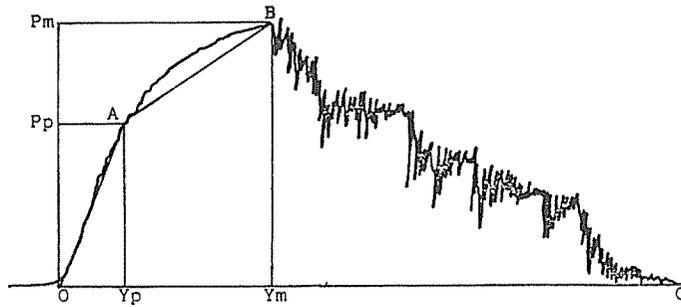
Fig. 5. An example of load-deflection curve
