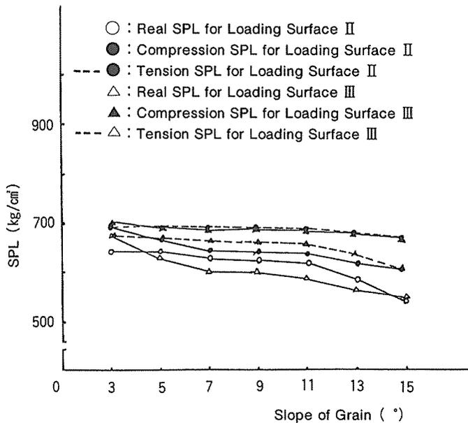
Fig. 8. Stress at the Proportional Limit for The Second Assumption
