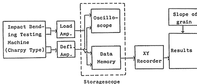
Fig. 4. A Flow Chart of the Data Recording.
