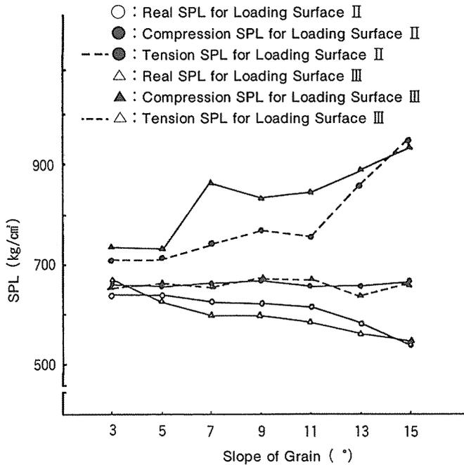
Fig. 7. Stress at the Proportional Limit for The First Assumption.
