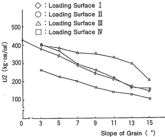
Fig. 16. Absorbed Energy from the Proportional Limit to the Fracture (U<sub>2</sub>) for Four Different Loading Surfaces.
