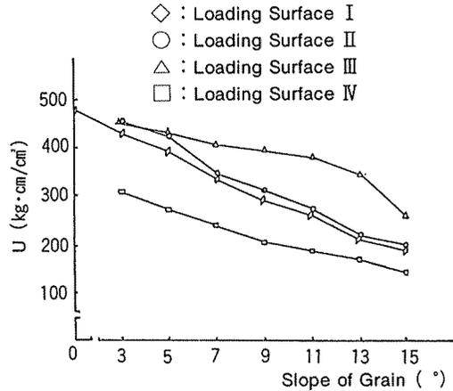
Fig. 17. Absorbed Energy to the Fracture (U) for Four Different Loading Surfaces.
