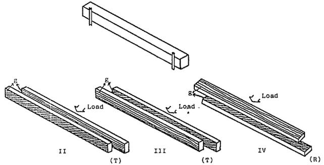
Fig. 2. Specimens & Loading Conditions II, III and IV.
