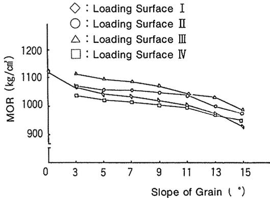
Fig. 9. Modulus of Rupture for Four Different Loading Surfaces.
