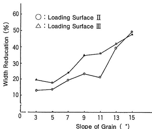
Fig. 6a. Percentage of Width Reduction in Stress at the Proportional Limit.
