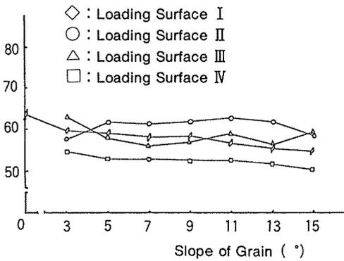
Fig. 15. Absorbed Energy to the Proportional Limit (U1) for Four Different Loading Surfaces.
