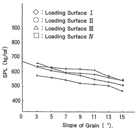
Fig. 6. Stress at the Proportional Limit for Four Different Loading Surfaces.
