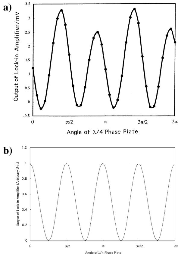
Fig. 3 Dependence of the output signal of the lock-in amplifier at the baseline upon the angle of the  $\lambda/4$  phase plate. a) Experimental results. b) Computer simulation.
