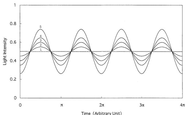
Fig. 2 Simulated sensor response. The phase shift at baseline ( $\Delta D = 0$ ) was set at  $D_0 = \pi/2$ . 1,  $\Delta D = 0$ ; 2,  $\Delta D = 0.1$ ; 3,  $\Delta D = 0.2$ ; 4,  $\Delta D = 0.3$ ; 5,  $\Delta D = 0.5$  (radian unit).
