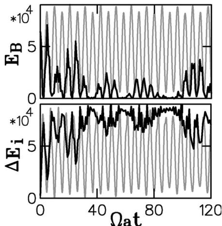
FIG. 4. Time variations of magnetic perturbation energies and ion kinetic energies,  $\Delta E_i = E_i - E_{i0}$ . The gray and black lines show energies in the single- and four-ion-species plasmas, respectively. The energies are normalized to  $m_e v_{Te}^2$ .
