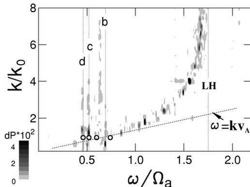
FIG. 8. An increase in  $P$ ,  $dP(k, \omega) = P_2(k, \omega) - P_1(k, \omega)$ , in the four-ion-species plasma. The four vertical lines represent the lower hybrid resonance frequency and heavy-ion cutoff frequencies.
