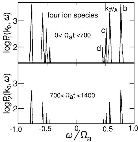
FIG. 7. The power spectra of magnetic fields with  $k=k_0$  in the four-ion-species plasma. The heavy-ion cutoff frequencies are  $\omega_{b0}/\Omega_a=0.69$ ,  $\omega_{c0}/\Omega_a=0.52$ , and  $\omega_{d0}/\Omega_a=0.46$ , while the frequency of the magnetosonic mode is  $k_0 v_A/\Omega_a=0.60$ .
