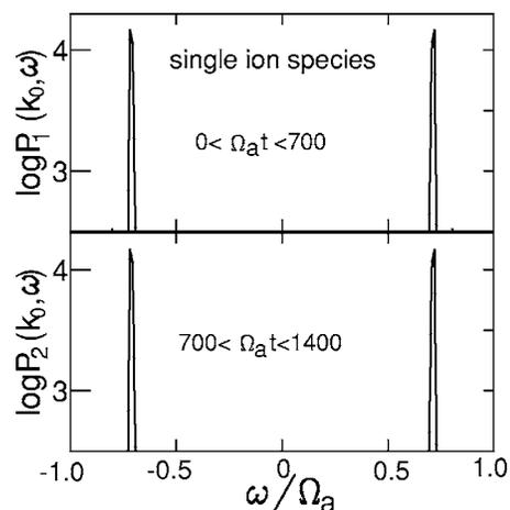
FIG. 6. Power spectra of magnetic fields with  $k=k_0$  in the single-ion-species plasma. The upper and lower panels are for the periods  $0 < \Omega_a t < 700$  and  $700 < \Omega_a t < 1400$ , respectively.
