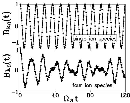
FIG. 3. Time variations of the Fourier component  $B_{k_0}(t)$  in the single- and four-ion-species plasmas. The dots and solid lines represent the simulation results and the theory, Eq. (4), respectively. The values of  $B_{k_0}(t)$  are normalized to its initial value  $B_{k_0}(0)$ .
