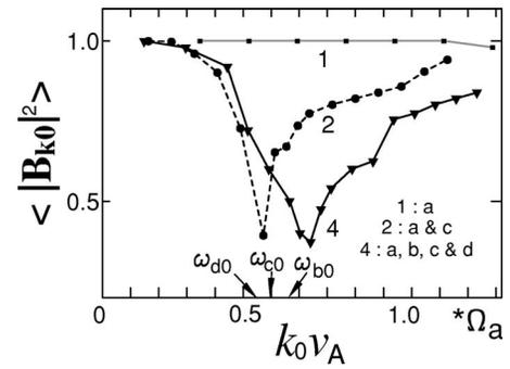
FIG. 12. Dependence of time-averaged  $|B_{k_0}(t)|^2$  on the wave number  $k_0$  and on the number of ion species. Here,  $\langle |B_{k_0}(t)|^2 \rangle$  for three cases (single-, two-, and four-ion-species plasmas) are shown.
