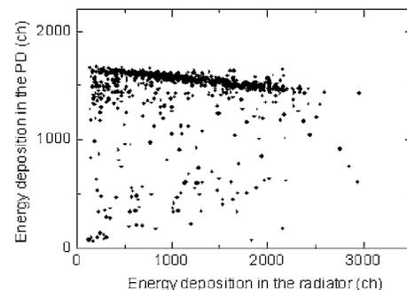
FIG. 3. The relation between the energy deposition of recoiled proton in the radiator and the PD.
