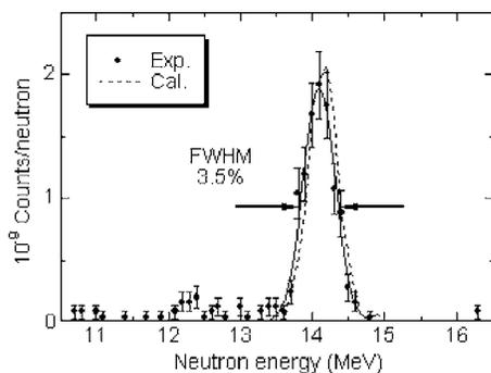
FIG. 4. DT neutron energy spectrum.
